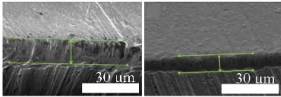
SEM-image of cutting edge of dental curette after wear
