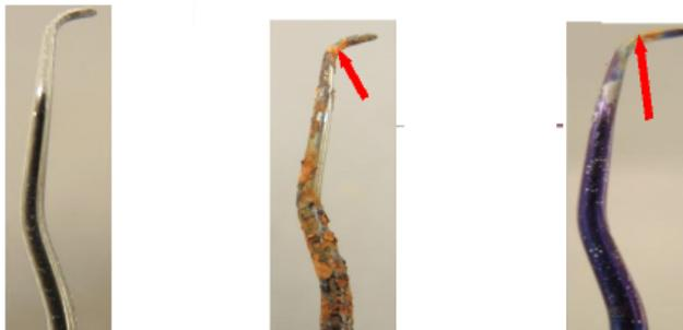
Photographs after 48 h in neutral salt spray test
