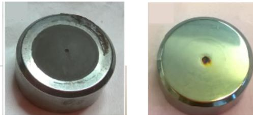
Photograph after corrosion testing (salt solution)
