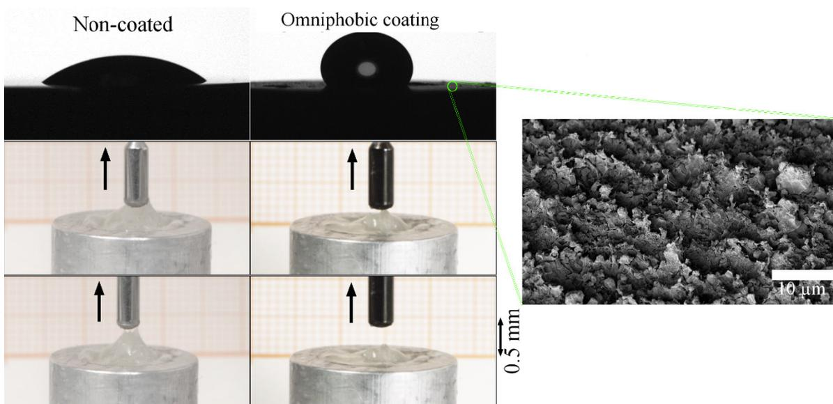
**Figure 2:** Left: non-coated restorative instrument. Middle: in-house fabricated omniphobic coated instrument. Right: SEM-image of textured surface, before coating deposition. Image taken from [III].
