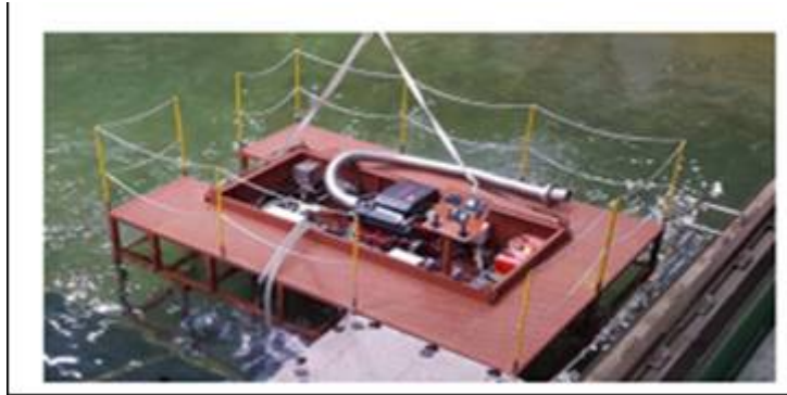
Figure 11: Basin Test of the USV Platform
