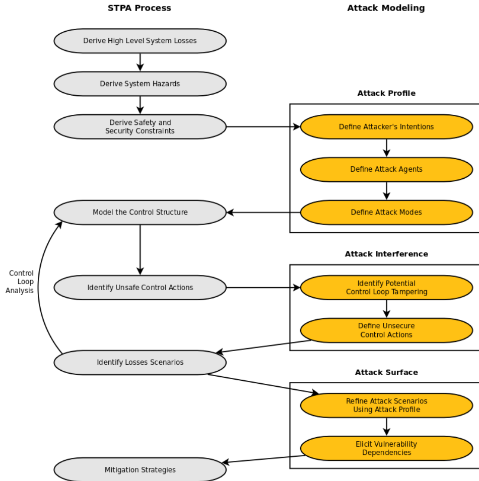
Figure 1: Extension of STPA Process (Leveson & Thomas, 2013) with Attack Modeling
