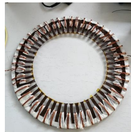
Figure 1: Ring core assembled from the stator laminations.
