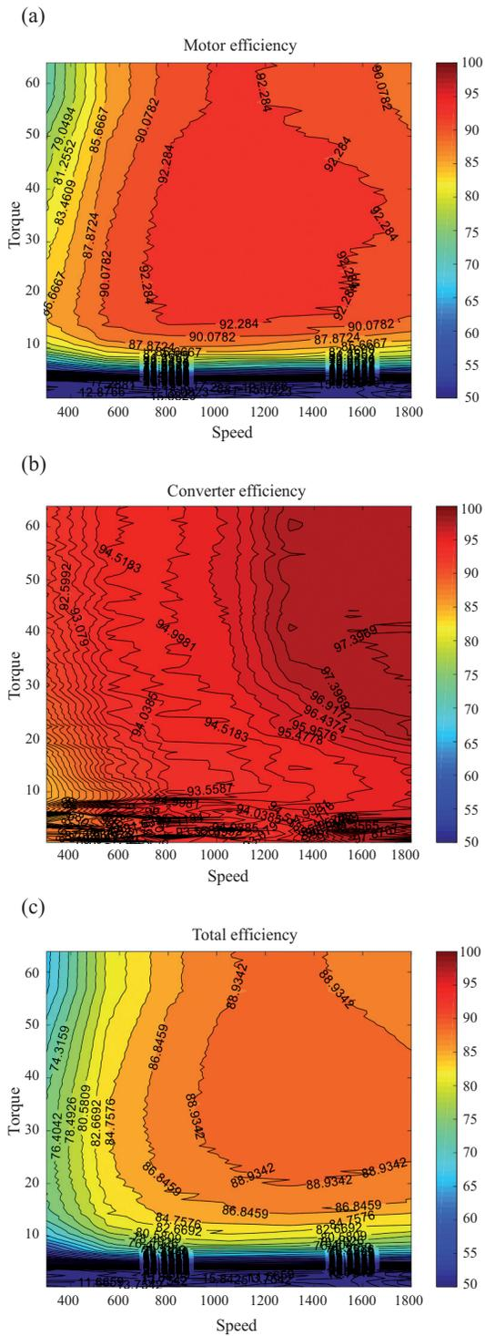
**Fig. 4.** Efficiency maps of the studied PMSynRM (a), feeding PMSynRM frequency converter (b), and the whole PMSynRM motor-drive system (c).
