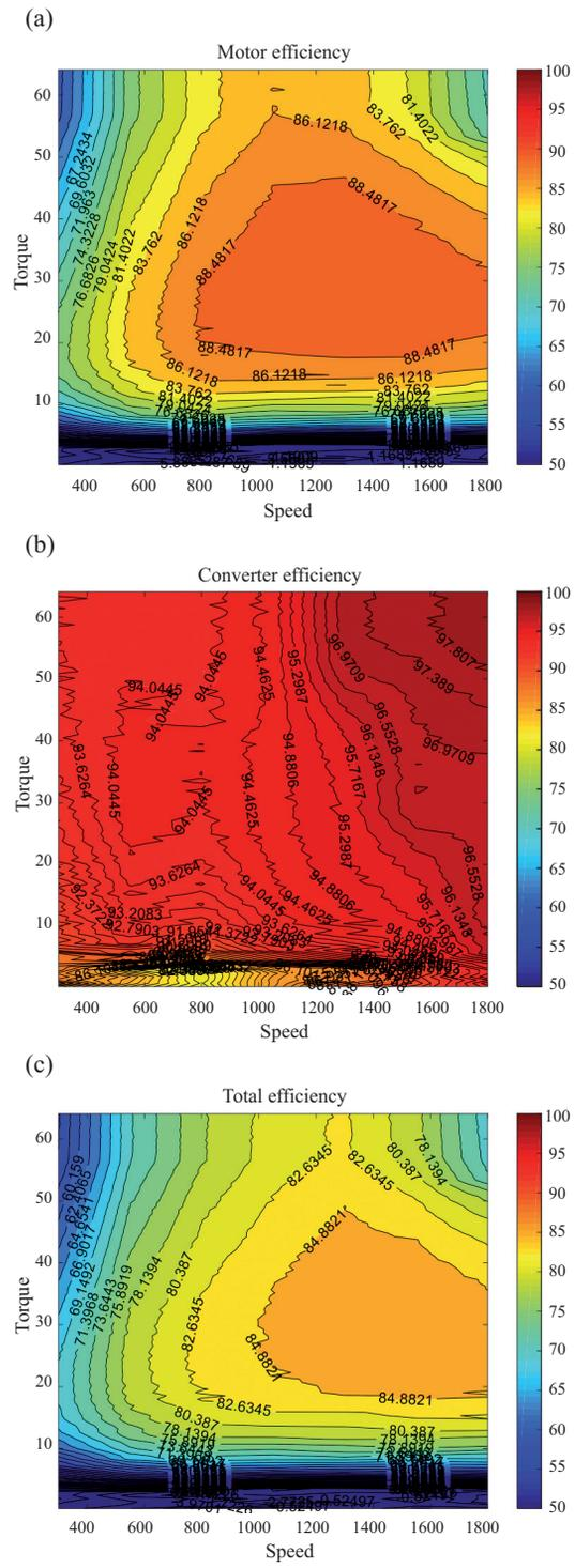
**Fig. 5.** Efficiency maps of the studied IM (a), feeding IM frequency converter (b), and the whole IM motor-drive system (c).
