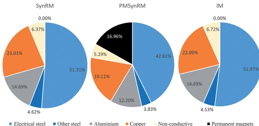
Fig. 7. Percentage ratio of raw material price based on different 10 kW motors production.
