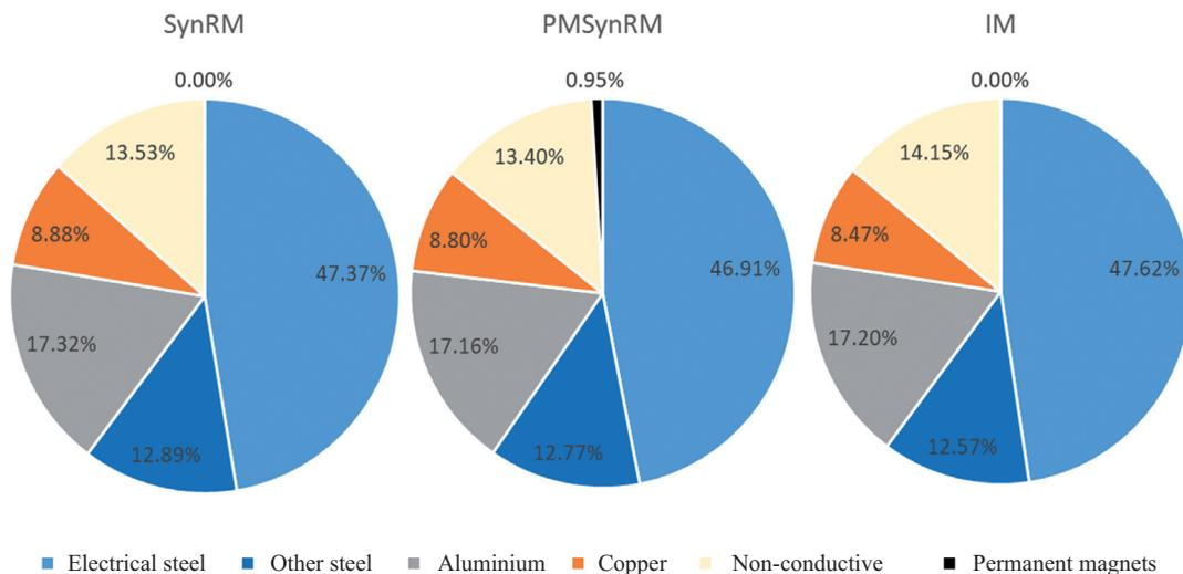
**Fig. 1.** Percentage ratio of raw materials used for different 10 kW motors production.
