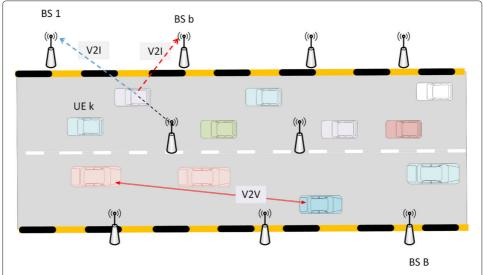
Fig. 1  $\,^{\circ}$ 2I and  $\,^{\circ}$ 2V communication system with  $\,^{B}$  BSs. A  $\,^{\circ}$ 2V/V2I example; a UE communicating with three mMIMO BSs and direct communication between a pair of UEs
