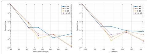
**Fig. 11** Relative mean-square error of prediction  $\delta^2_{\mathcal{P},g}$  (left plot) and  $\delta^2_{\mathcal{C},g}$  (right plot). The small values of  $\delta^2_{\mathcal{P},g}$  and  $\delta^2_{\mathcal{C},g}$  indicate that the LQP model provides reliable prediction of the outage probability of the out-of-sample UEs
