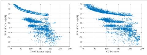
$\textbf{Fig. 9} \ \ \text{Scatter plot of the average SNR of V2V links as a function of true distance (left plot) and CC distance (right plot)$
