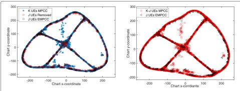
**Fig. 8** Two-dimensional channel chart for 10 BSs. The channel chart location of out-of-sample UEs is in black color. Left: re-inserting removed sample. Right: inserting new sample
