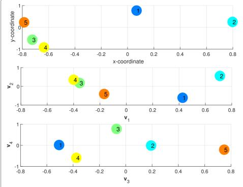
**Fig. 2** A connected graph of five nodes. Top: two-dimensional true location of the nodes. Middle: LE logical location of the nodes using the first and second Eigenvectors. Bottom: logical location using the third and fourth Eigenvectors
