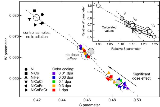
**Fig. 3.** (S, W) parameters of the irradiated samples, the large empty circle represents the center-of-mass of the control samples. The inset shows theoretical predictions for different sizes of vacancies in the NiCoFeCr systems. The dashed lines in the figure and the inset represent the same slopes. The error bars are at most the size of the markers.
