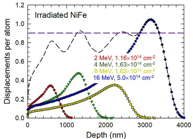
**Fig. 1.** SRIM-predicted dpa profile for the NiFe sample, assuming the density of 8.232 g cm<sup>-3</sup>, irradiated with multiple energies of Ni ions. The Ni energies and the corresponding fluences are indicated on the plot. The purple dashed line represents the average dpa level for this irradiation sequence, corresponding to an average Ni concentration of  $3 \times 10^{18}$  cm<sup>-3</sup>.
