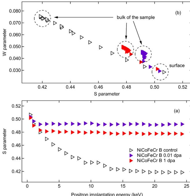
**Fig. 2.** (a) S parameter measured as a function of the positron implantation energy in selected samples. (b) (S, W) parameters for the same samples, the positron implantation energy is the running parameter in the data points. The error bars are at most the size of the markers.
