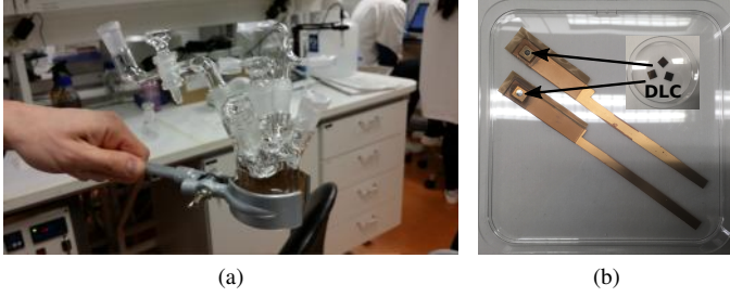
Fig. 11. Dopamine solution and sensor electrode preparation: DLC samples are attached to copper contact strips which enables connection of the electrodes to the measurement board.
