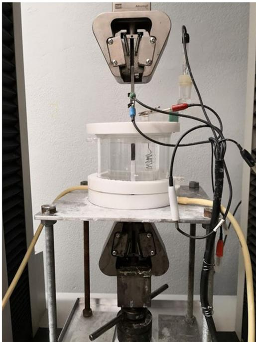
**FIGURE 3** The tensile testing system consisting of a 35 kN MTS desktop machine with an electrochemical cell and Gamry potentiostat [Color figure can be viewed at [wileyonlinelibrary.com](http://wileyonlinelibrary.com)]
