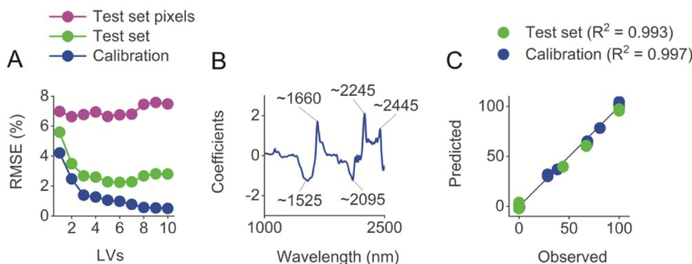
**Fig. 3.** Initial image calibration. Root mean squared errors (RSME) based on the average calibration and test set spectra and the individual test set pixels as a function of latent variables used in the model (A), the regression vector on 2 latent variables (B) and the predicted vs. observed PET contents (%) based on 2 latent variables (C).
