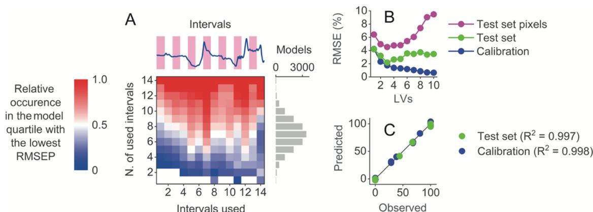
**Fig. 4.** Variable selection and image calibration. Relative occurrence of individual intervals in the model quartile with the lowest RMSEP during variable selection (A), average prediction errors with intervals 5, 6, 7, 10 and 12 as a function of latent variables (B), and the predicted and observed polyester contents (%) based on three latent variables (C).
