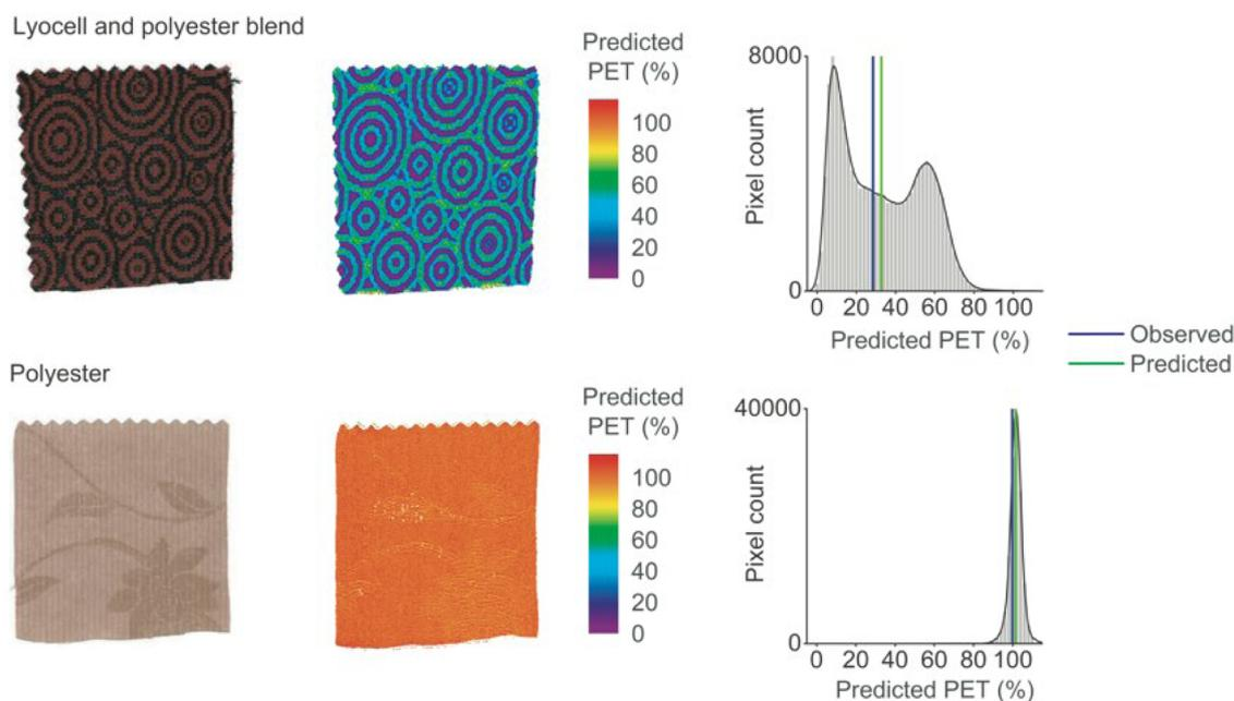
**Fig. 5.** Image predictions. Two textile samples (left), their polyester contents based on image predictions (middle) and the respective pixel histograms which illustrate the distributions of the predicted pixel values (right). The histograms have different vertical scales and the colored vertical lines denote the mean observed and predicted values. The reader is referred to the electronic version of this article for proper illustration of figure colors.
