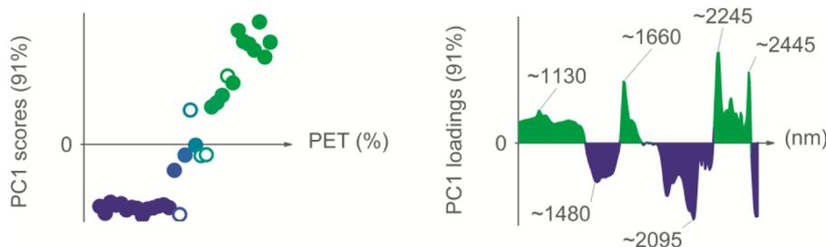
**Fig. 2.** Exploratory data analysis. Sample scores on the first principal component (left) and the respective loadings (right) based on the average spectra of the samples. The scores were sorted according to increasing polyester (PET) contents in the samples and the unfilled symbols were deemed as outliers and excluded from further image calibration. The numbers in the loadings denote wavelength values in nanometers.
