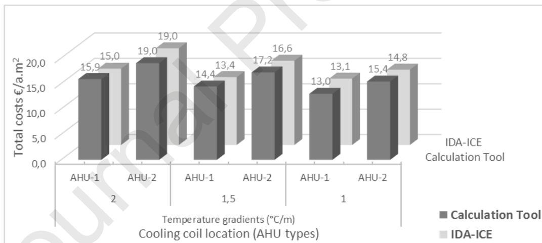
Fig. 20. Cooling coil location effects on total costs calculated by the tool compared with IDA-ICE (€/m<sup>2</sup>.a).
