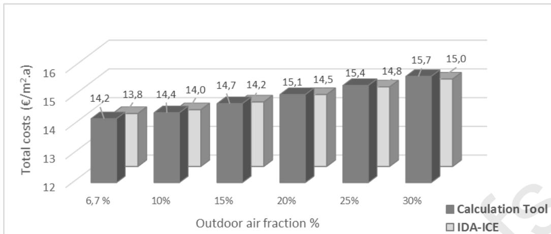
Fig. 19. Outdoor air fraction effects on total costs calculated by the tool compared to IDA-ICE (€/m<sup>2</sup>.a).
