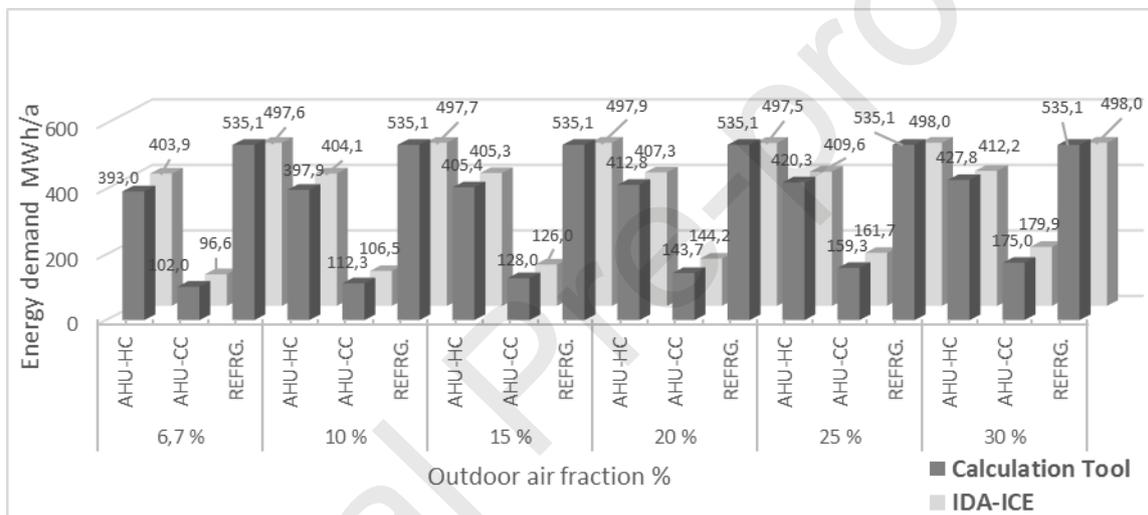
Fig. 18. Outdoor air fraction effects on energy consumption calculated by the tool compared to IDA-ICE (MWh/a).
