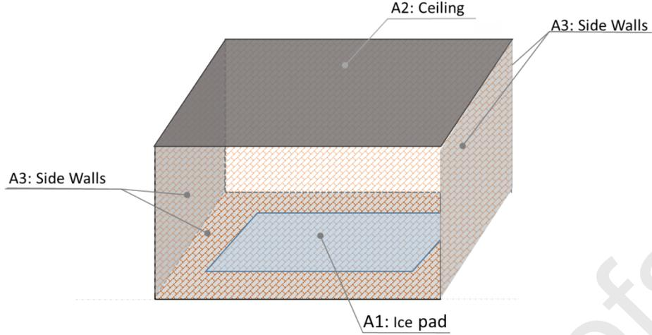
Fig. 5. Ice rink model for calculating the radiation heat transfer.
