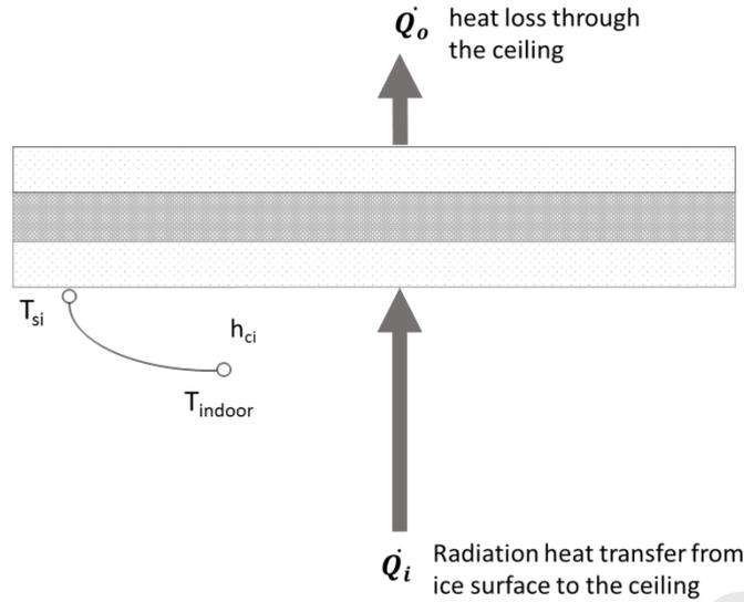
Fig. 7. Thermal analysis for ceiling surface temperature calculation.
