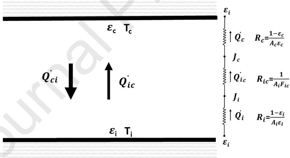
Fig. 6. Two-surface enclosure and its electrical network model.
