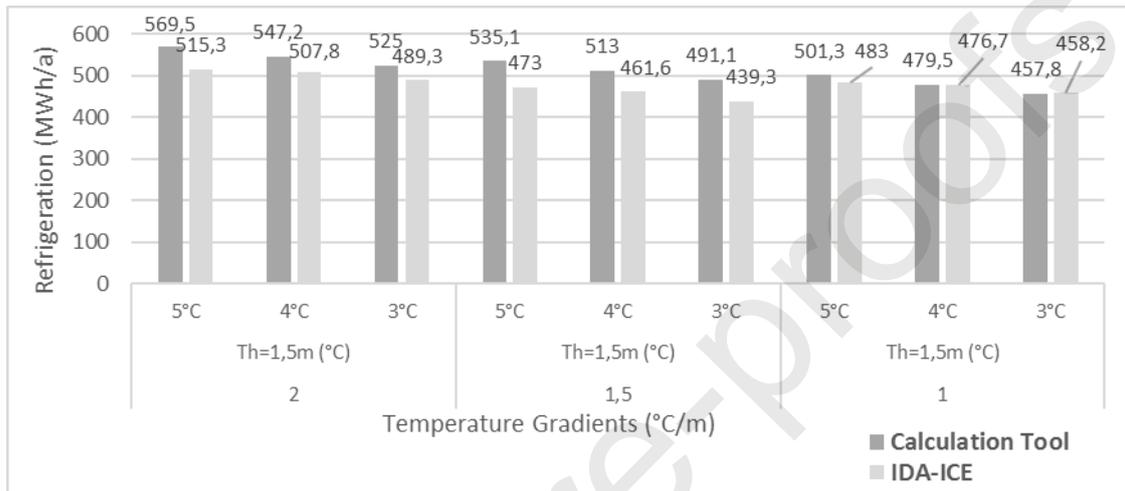
Fig. 16. Comparison of refrigeration demand of IDA-ICE with the calculation tool (MWh/a).
