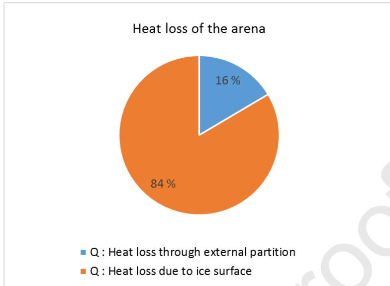
Fig. 9. Contribution of external partitions and internal loads to overall heat loss.
