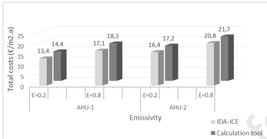
Fig. 21. Emissivity effects on total costs calculated by the tool compared with IDA-ICE (€/m<sup>2</sup>.a).
