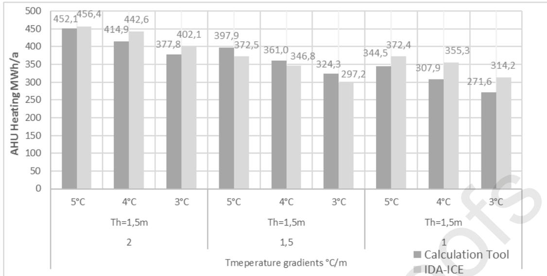
Fig. 14. AHU heating demand results of IDA-ICE compared with the calculation tool results (MWh/a).
