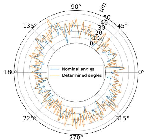
**Fig. 8.** Effect of correcting the angles on roundness profile calculated from measured data from the roll. The nominal and incorrect angles used in the calculation are shown in Table 1.
