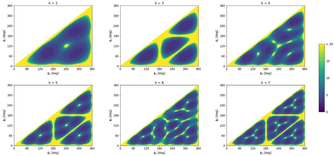
**Fig. 4.**  $\kappa_k$  calculated separately for single harmonics  $k = 2, \dots, 7$ , showing how each added harmonic results in added areas of suppression with the distance between the suppressed areas decreasing as the harmonic number increases. It can also be seen that odd harmonics are suppressed when at least one of the angles is equal to  $180^\circ$ . The final performance index  $T$  is a weighted sum of the single harmonics' indexes (Eq. (5)).
