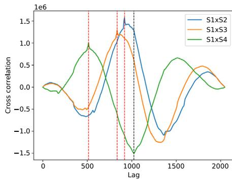
**Fig. 6.** One round (1024 samples) of measured signals cross correlated with each other. The red line shows the maximum, which is the probe position.
