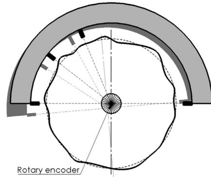
Fig. 3. Schematic picture of positioning error showing how a placement error of a fixed measurement frame results in altered probe angles.
