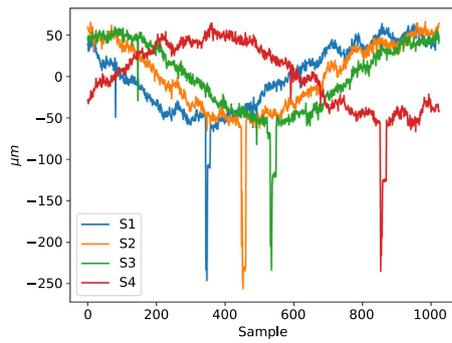
**Fig. 5.** One round (1024 samples) of measured displacement signals. The notches in the signals are caused by the marker.
