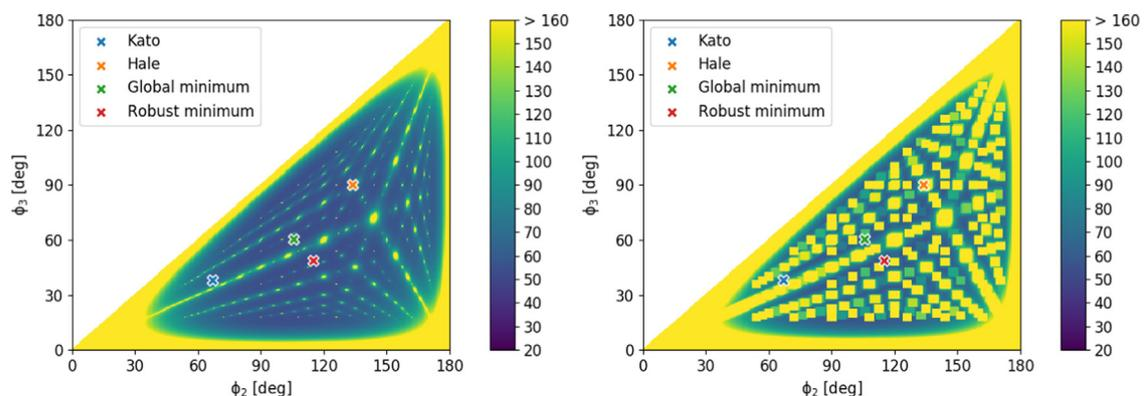
Fig. 9. On the left, performance index  $T$  (Eq. (5)) as a function of the probe angles with harmonics  $2, \dots, 20$  with linearly decreasing weighting  $h_k$ . The robust optimization (Eq. (6)) is shown on the right.
