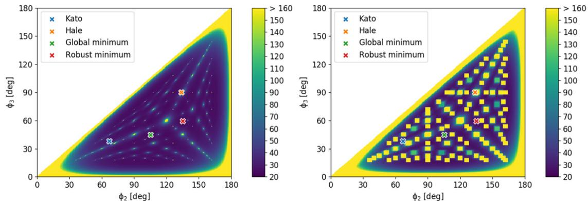
**Fig. 10.** On the left, performance index  $T$  (Eq. (5)) as a function of the probe angles with only odd harmonics in the range  $2, \dots, 20$  with linearly decreasing weighting  $h_k$ . The robust optimization (Eq. (6)) is shown on the right. The results of this optimization are intended for a redundant roundness measurement method, where even harmonics are calculated from a diameter variation profile.
