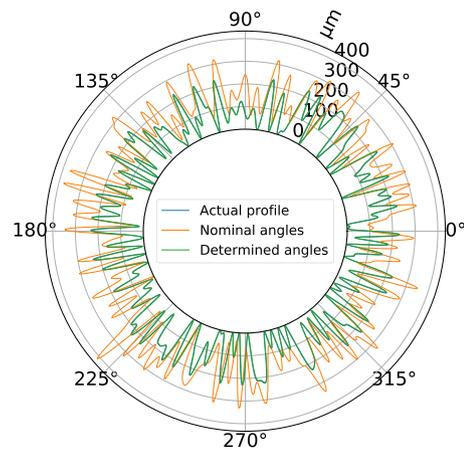
**Fig. 7.** Roundness profile calculated from simulated signals with incorrect angles and determined corrected angles. The nominal and incorrect angles used in the calculation are shown in Table 1.
