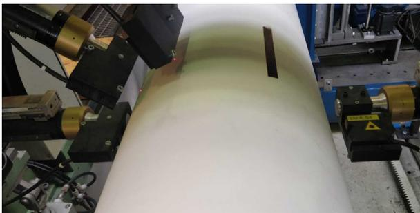
Fig. 2. Measurement setup with rotor, marker and four laser sensors.
