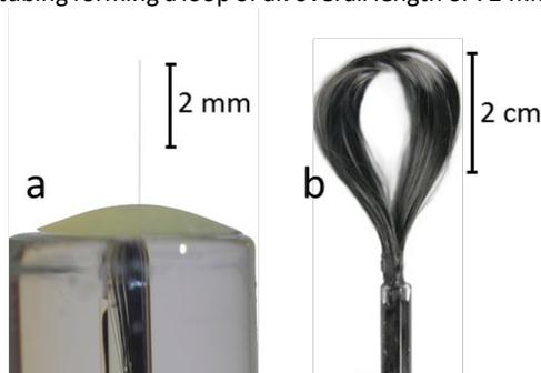
**Fig. 2.** CF electrodes used in this work: a) carbon fibre microcylinder electrode (CFMCE), b) carbon roving loop electrode (CRLE).
