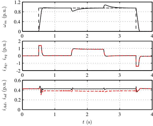
Fig. 7. Simulation results showing speed and load changes. The first subplot shows the rotor speed (solid), its reference (dashed), and its estimate (dotted). The second subplot shows the  $q$ -axis components of the stator current (solid) and the inverter output current. The third subplot shows the  $d$ -axis components of the stator current (solid) and the inverter output current.
