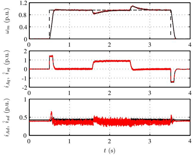
Fig. 9. Experimental results showing a sequence with speed and load changes. The explanations of the curves are as in Fig. 7. Estimated values are shown for the stator current.
