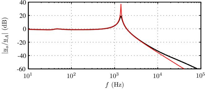
Fig. 3. Amplitude-frequency response from  $\underline{u}_A$  to  $\underline{u}_s$  when frequency-dependent inductor model is used (thick line) and when inductor parameters are constant:  $L_f = L_{f,dc}$  and  $R_{L_f} = R_{L_f,dc}$  (thin line).
