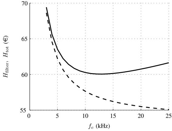
Fig. 6. Cost as function of switching frequency. Dashed line is the filter component cost  $H_{\text{filter}}$ . Solid line is the total cost of the filter components and inverter oversizing.
