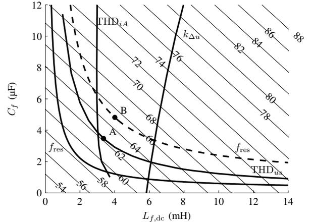
Fig. 5. Optimal filter design. Point A is the optimal design if  $f_{\text{sa}} = 2f_c$ . Point B is the optimal design if  $f_{\text{sa}} = f_c$ .
