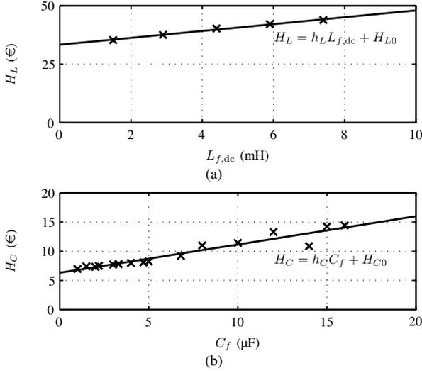
Fig. 4. Filter component prices: (a) Three-phase inductor (5 A), (b) Capacitor (450 V). Price parameters are  $h_L = 1.47$  €/mH,  $H_{L0} = 33.3$  €,  $h_C = 0.48$  €/μF, and  $H_{C0} = 6.3$  €.
