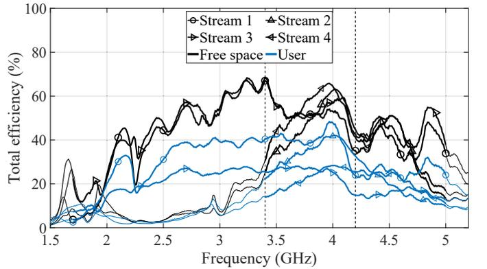
Fig. 10. Measured high-band total efficiency for Case II version 2 antenna.
