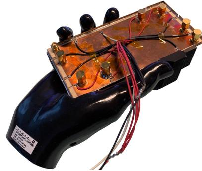
Fig. 2. The measured antenna prototype for Case I and the hand phantom used in the measurements.
