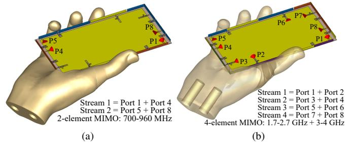
Fig. 1. (a) Low-band operation and (b) high-band operation port configurations and operation bands for the antenna of Case I. The elements of every antenna cluster are marked with same color.
