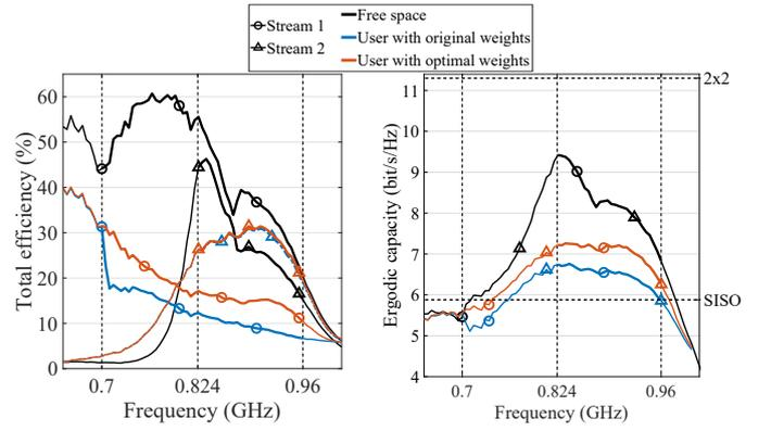
Fig. 8. Measured total efficiencies and calculated capacities for the low-band antennas for Case II.
