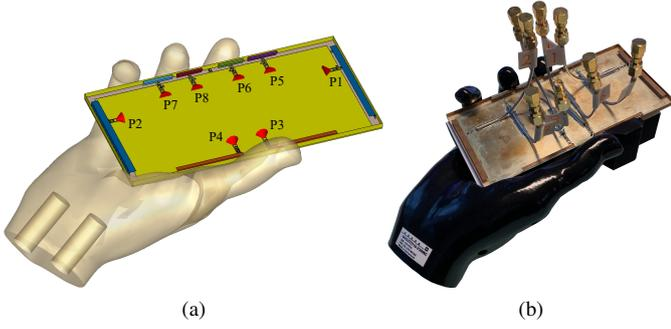
Fig. 7. (a) Antenna model and (b) measured prototype with the hand phantom for Case II.
