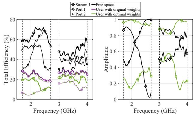
Fig. 5. Efficiencies of the antenna cluster and the individual elements and the amplitudes of the feeding weights in free space and with the user for Case I high-band.
