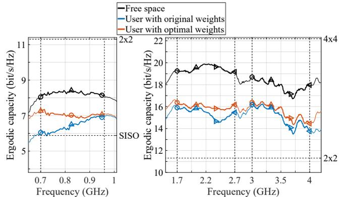
Fig. 6. Capacities calculated for the low-band and high-band results in free space and with the user for Case I.
