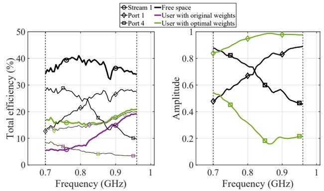
Fig. 4. Efficiencies of the antenna cluster and the individual elements and the amplitudes of the feeding weights in free space and with the user for Case I low-band.
