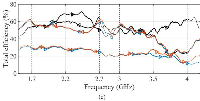
Fig. 3. Measured total efficiencies in free space and with user for Case I for (a) low band, (b) high band streams 1 and 2, and (c) high band streams 3 and 4.
