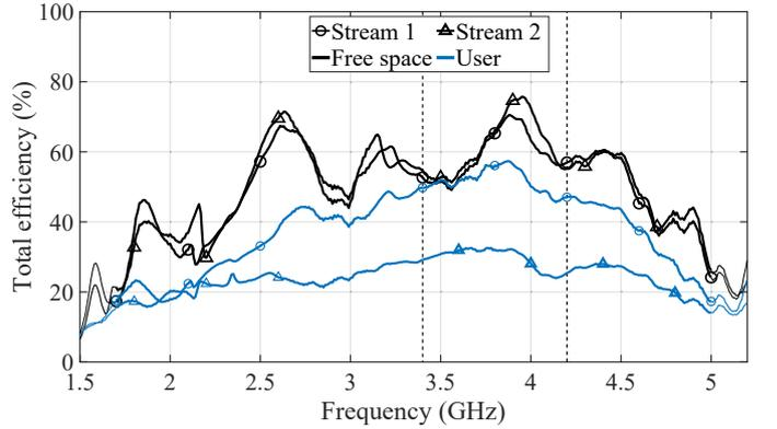
Fig. 9. Measured high-band total efficiency for Case II version 1 antenna.
