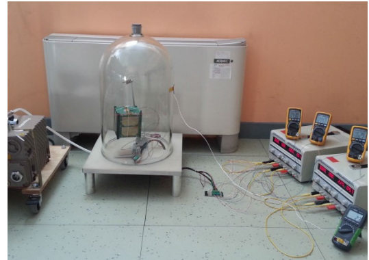
FIGURE 17. Absorption co-efficient measurement setup.
