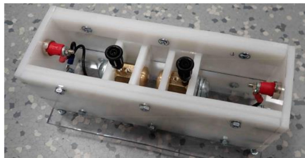
Figure 9. Adjustable sphere–sphere spark gap [33].
