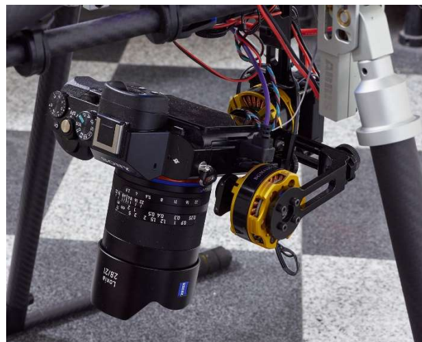
Figure 1. The 3-axis gimbal and the Sony Alpha 7R camera system with the Zeiss Loxia 2.8/21 lens.
