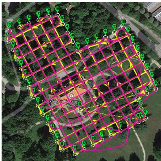
Figure 11. Flight plan and realised flight path of an example survey mission in Träskända. Planned flight path is shown in yellow and the drone flight path is illustrated in magenta.
