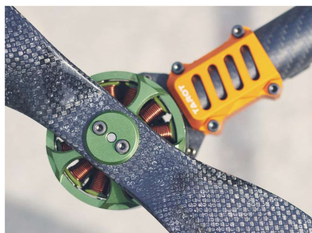
Figure 3. Multistar Elite 5008-330 fitted with a 18” 5.5” pitch propeller and attached to a Tarot T960 hexacopter frame. © Aalto University
