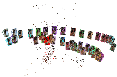
Figure 7. Imaging geometry of the second test case. Imaging geometry is not as strong as in the first test case because images were taken along a nearly horizontal trajectory.
