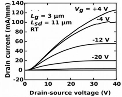
**Figure 4:** Output characteristics of N-polar PolFET with a 30-nm-thick  $Al_2O_3$  gate dielectric.
