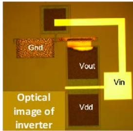
**Figure 5:** Optical image of a complementary logic GaN inverter fabricated on a GaN-on-Si platform.
