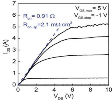
**Figure 1:** Output characteristics and extracted  $R_{on}$  and  $R_{sp,on}$  in a vertical GaN power FinFET.
