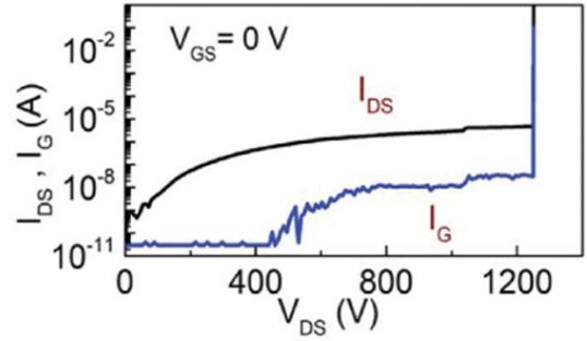
**Figure 2:** Off-state leakage of a vertical FinFET measured at  $V_{GS} = 0V$ , demonstrating a breakdown voltage of 1250 V.
