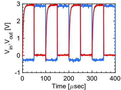
**Figure 6:** Transient response of the GaN complementary logic inverter shown in Figure 5.
