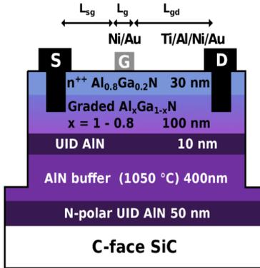
**Figure 3:** Schematic cross-section of the fabricated N-polar AlGaN/AIN PolFET with recessed contacts.
