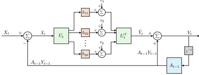
**Fig. 2:** Feedback realization of the optimal reproduction process by parallel channels for multivariate Gaussian sources.
