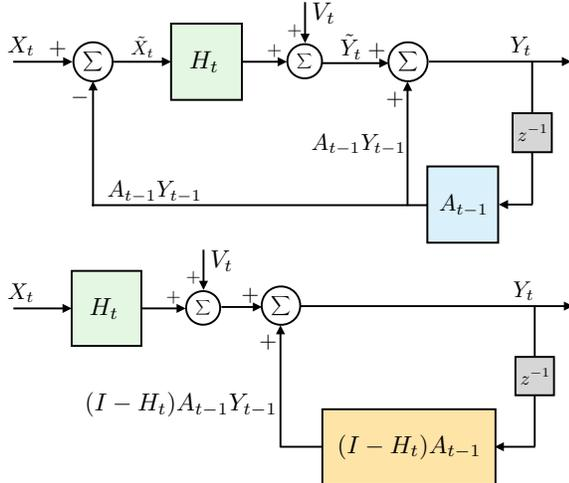
**Fig. 1:** Equivalent Realizations-Block diagrams of two realizations for multivariate Gaussian sources with feedback (top) and without feedback (bottom). The realization with feedback is coming from (26)-(28), while the one without feedback from (16).
