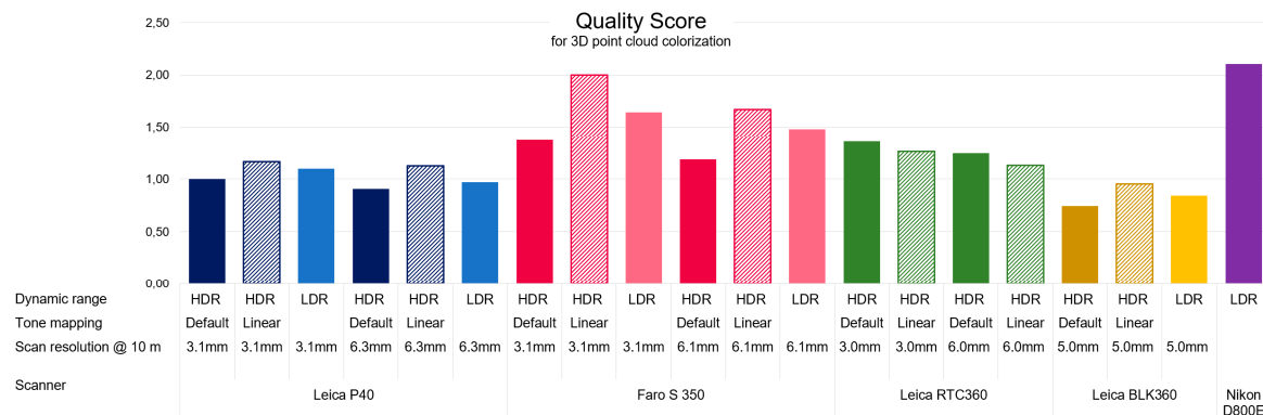
Figure 13. Quality score combining the selected image quality metrics into one 3D point cloud colorization quality score for all tested scans and the photographic reference.
