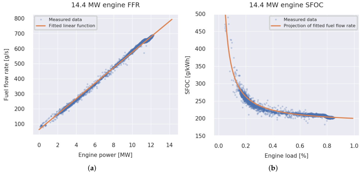
Figure 5. Large engine measured fuel flow rates and linear fuel flow rate curve fit (a) and linear fuel flow rate function projection on engine SFOC curve (b).
