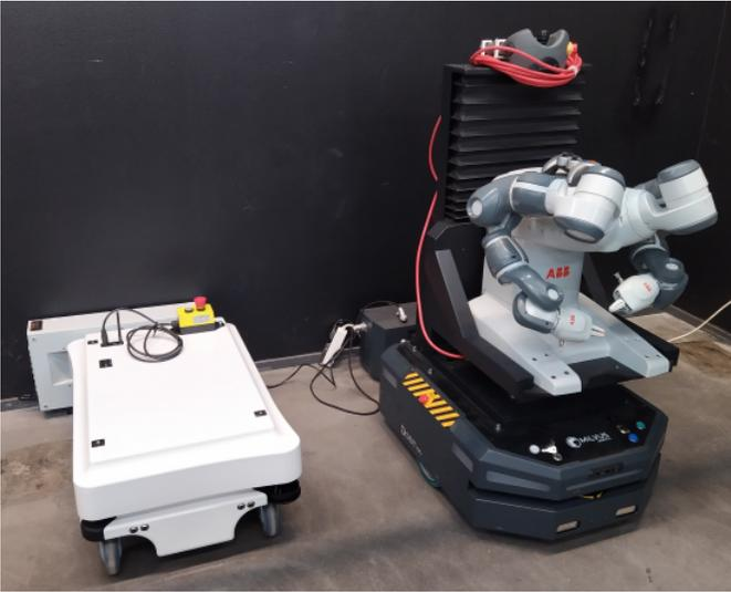
Fig. 3. Industrial AGVs at the Aalto Factory of the Future
