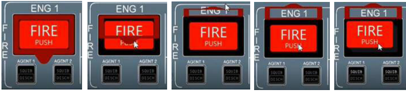
Fig. 4: Interactions sequence for pushing overhead panel-like FIRE push button.
