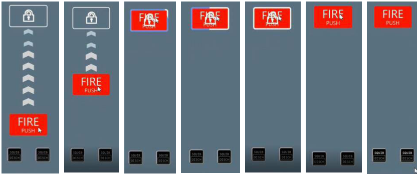
Fig. 5: Interactions sequence for pushing GoPro-like FIRE push-button.
