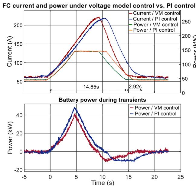
Fig. 10. Power cycling test between the proposed voltage model (VM) controller and the PI controller from [12].
