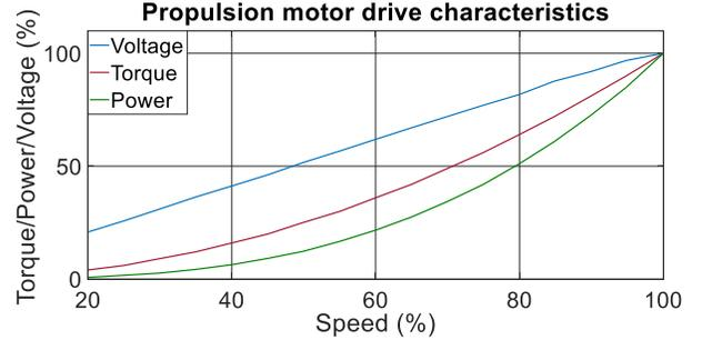
Fig. 3. Characteristics of a propulsion motor drive. Nominal torque and speed of the motor are 2040 Nm and 1480 rpm, respectively.
