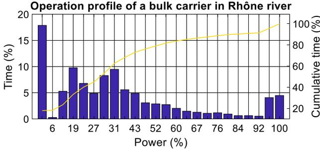
Fig. 1. Operational profile of a bulk carrier in Rhône river [15]. The bars show load power distribution in a single trip. The curve shows cumulative load distribution.
