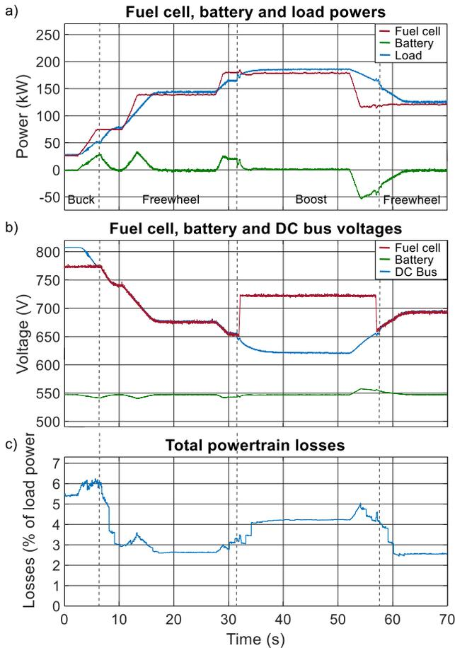
Fig. 14. a) Power, b) voltage and c) losses of drivetrain components during different operating modes when operated with variable DC Approach. Optimal efficiency is achieved in Freewheel mode.
