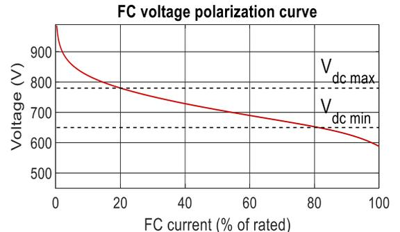
Fig. 4. An FC polarization curve, where  $V_{dc\_min}$  and  $V_{dc\_max}$  are minimum and maximum DC bus operation voltages, respectively.
