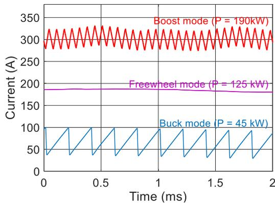
Fig. 15. HF current ripple at the FC output. In Freewheel mode, the HF ripple is filtered by the DC bus capacitors and the inductor of FC converter.
