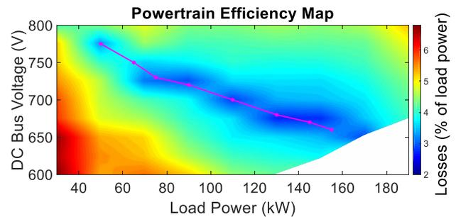
Fig. 13. Total drivetrain efficiency map as function of power and DC bus voltage.
