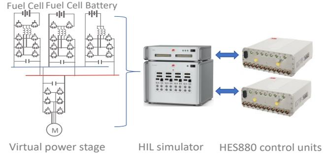
Fig. 8. A HIL test setup consisting of two FC units, a battery unit and a propulsion motor unit.
