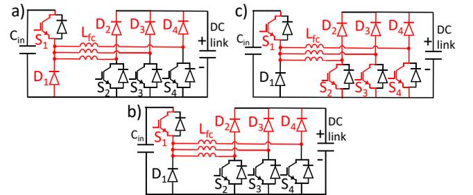
Fig. 9. FC converter diagram and its operation modes: a) Buck mode ( $S_1$  in PWM,  $S_2$ - $S_4$  off), b) Freewheeling mode ( $S_1$  constantly on,  $S_2$ - $S_4$  off) and c) Boost mode ( $S_1$  constantly on,  $S_2$ - $S_4$  in PWM). [12]
