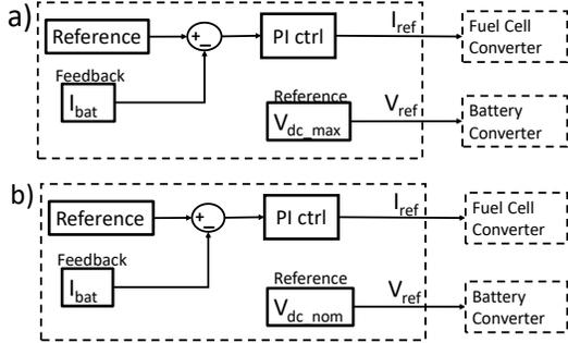
Fig. 6. Control of FC current in a) Buck mode and b) Boost mode. Battery voltage reference is fixed at maximum value and nominal value in Buck and Boost modes, respectively. [12]
