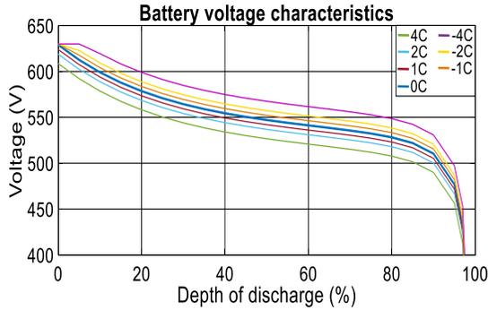
Fig. 5. Battery voltage characteristics as function of SOC and current.
