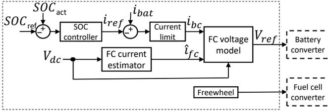
Fig. 7. A high-level diagram of the proposed voltage controller in Freewheel mode.
