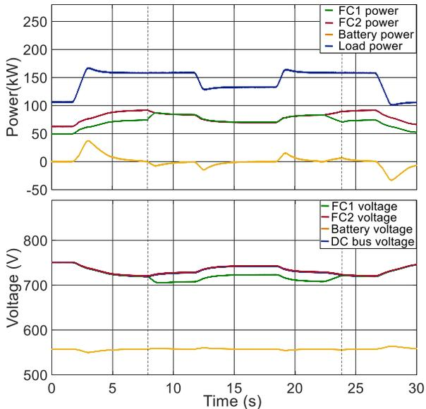
Fig. 12. Control of two differently rated fuel cells in Freewheel mode. Between the dashed vertical lines, the more degraded FC is set to Boost mode to force equal load sharing.
