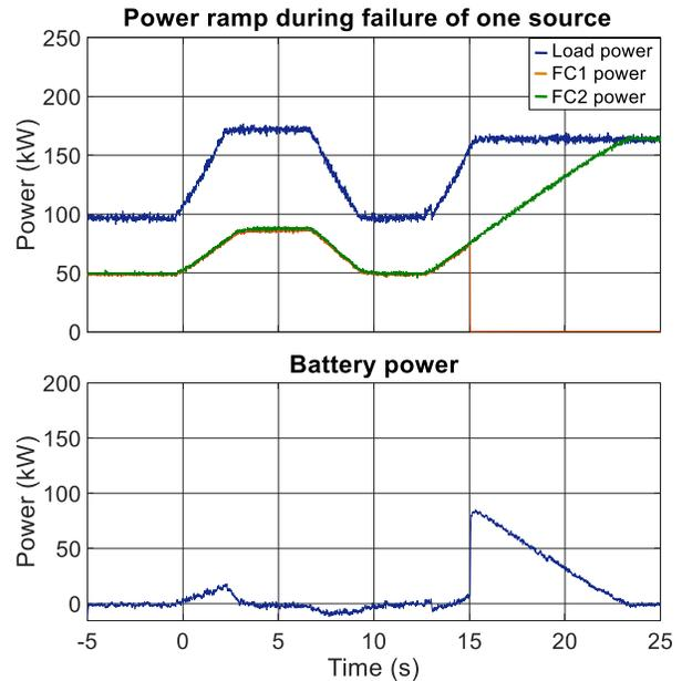
Fig. 11. A power failure test using two FCs. At 15s, FC1 is tripped but operation of the rest of the system is continued.
