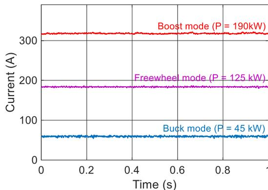
Fig. 16. LF current ripple at the FC output. No significant difference can be noticed in the current ripples between different modes. The maximum LF peak to peak ripple values are ca. 7.5A, 5.5A and 5.8A for Buck, Freewheel and Boost modes respectively.
