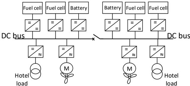
Fig. 2. An FC powered marine vessel system with DC distribution. Apart from propulsion, all other load (e.g., lighting and air conditioning) is considered hotel load.
