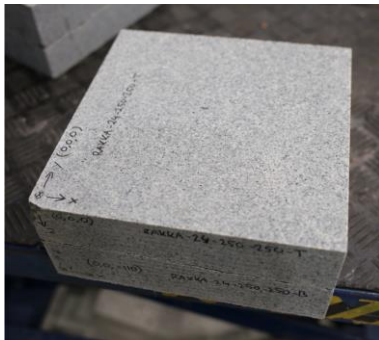
Fig. 1. Kuru gray granite slab pair 250 mm x 250 mm x 110 mm.
