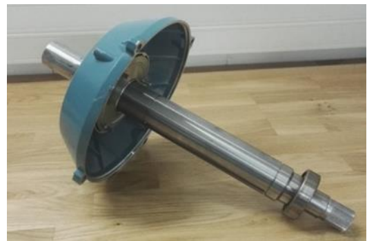
Fig. 10. Replacement of the rotor of SynRM with the shaft.
