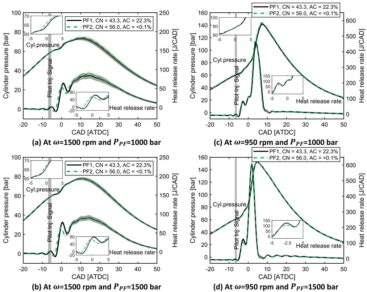
Fig. 9. Averaged cylinder pressure and heat release rate (HRR) data along with standard deviation at two different  $\omega$  and  $P_{PF}$ . Two pilot fuels (PF1 and PF2) are compared to study the combined effect of CN and AC on lean ( $\phi_{CH4} = 0.52$ ) DF combustion.
