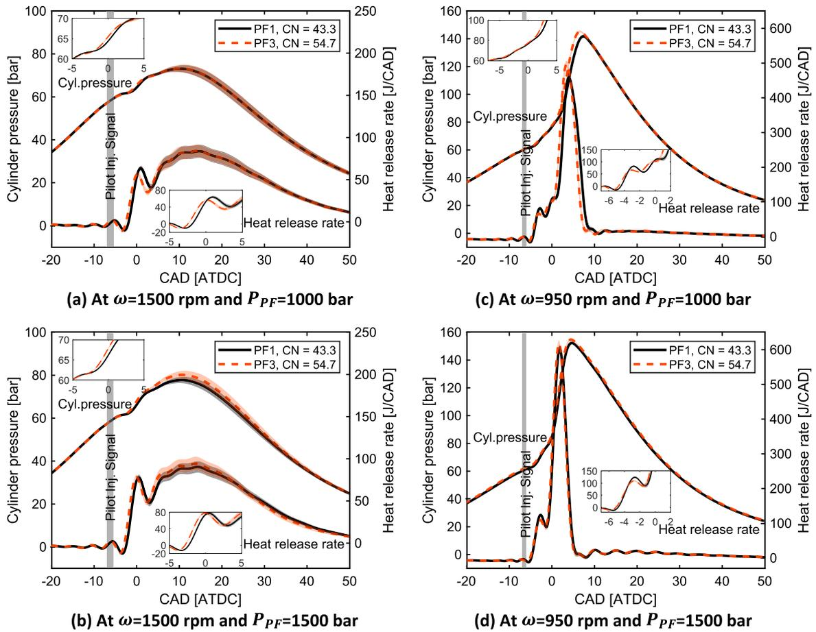
Fig. 3. Averaged cylinder pressure and heat release rate (HRR) data along with standard deviation at two different  $\omega$  and  $P_{PF}$ . Two pilot fuels (PF1 and PF3) are compared to study the effect of CN on lean ( $\phi_{CH_4} = 0.52$ ) DF combustion.
