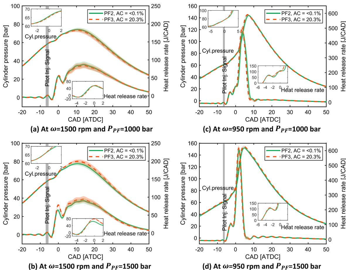
Fig. 6. Averaged cylinder pressure and heat release rate (HRR) data along with standard deviation at two different  $\omega$  and  $P_{PF}$ . Two pilot fuels (PF2 and PF3) are compared to study the effect of AC on lean ( $\phi_{CH_4} = 0.52$ ) DF combustion.
