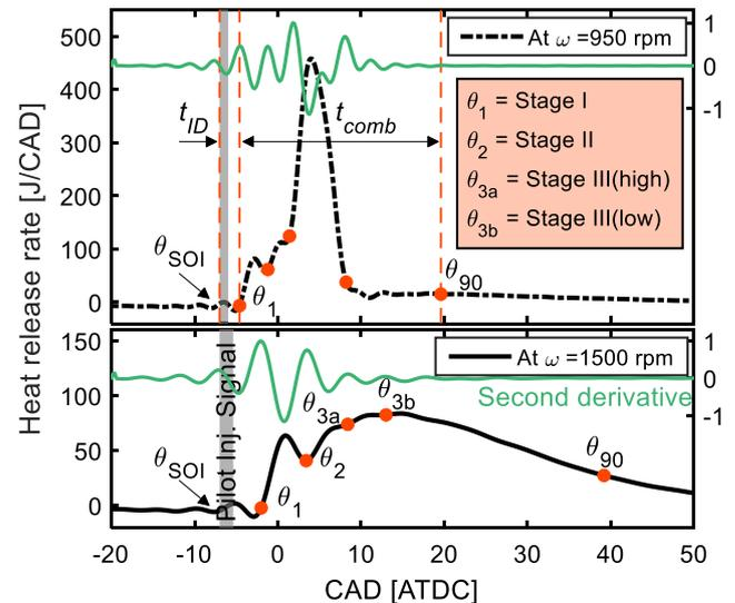
**Fig. 2.** An example showing the three overlapping DF combustion stages determined from typical HRR profiles investigated in this work. The stages are identified by the second derivation of HRR analysis. It is interesting to note that the profiles of the HRR curves tend to change from multi-peaks (M-shaped) to quasi-single peak with decreasing  $\omega$  from 1500 rpm to 950 rpm.
