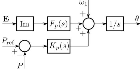
Fig. 3. Hybrid synchronization controller, merging PLL and PC.
