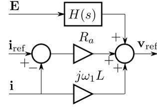
Fig. 2. CC with proportional part,  $dq$  decoupler, and PCC-voltage feedforward.
