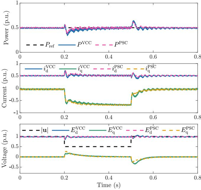
Fig. 9. Fault ride-through for SCR = 1 and  $\alpha_c = 8$  p.u.
