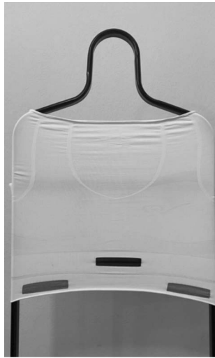
Fig. 2 - Piezoresistive sensors manufactured into flexible textile
