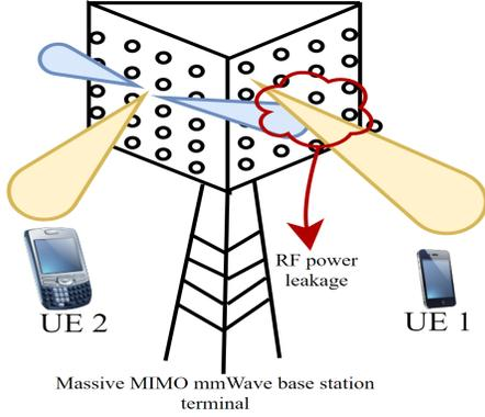
Fig. 1. Hybrid beamforming mmWave network model under RF power leakage constraint by using SDMA to separate users.
