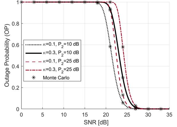
Fig. 3. Outage probability curves versus receive SNR for different levels of transceiver distortion noise and UE 2 average power.
