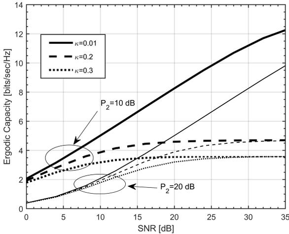
Fig. 5. Ergodic capacity for a hybrid beamforming mmWave network model under RF power leakage constraint and transceiver distortion parameters  $\kappa = 0.01; 0.2; 0.3$ .
