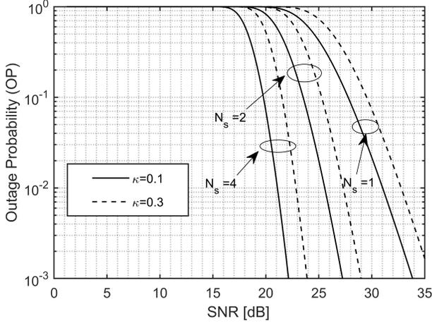
Fig. 4. Outage probability for a hybrid beamforming mmWave network model for  $L = 50$  m and different levels of transceiver distortion noise.
