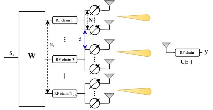
Fig. 2. Hybrid beamforming network with maximum sub-array transmission diversity technique directed to UE 1.
