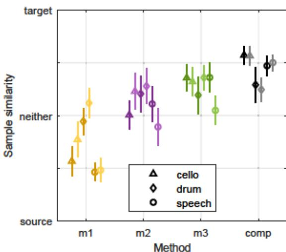
Figure 5: Marginal means and 95% confidence intervals ( $N = 13$ ) for interaction between *room*, *stimulus*, and *method* in the listening test. Each method is plotted with the same hue as in Figure 2, while the brightness of the color refers to different rooms. Finally, the marker indicates the stimulus used for that particular test sample.
