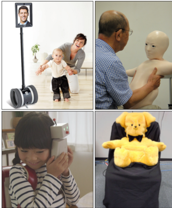
Figure 2: Telepresence Robots. Left to right: Double Robotics 2 , Telenoid (Ogawa et al., 2011), BOCCO 3 , stuffed-bear robot (Kuwamura et al., 2012).
