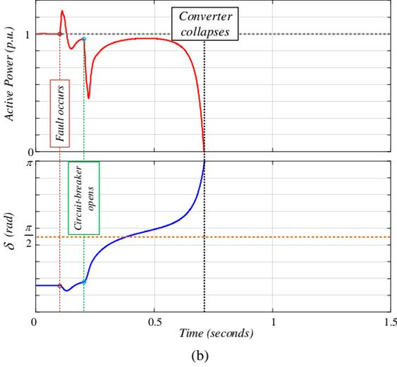
Fig. 4. (a) Phase portrait of conventional PSC. (b) Active power and power angle trajectory of conventional PSC following a solid fault.
