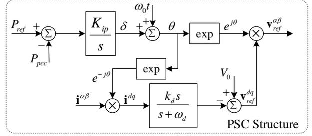
Fig. 1. Block diagram of PSC structure.
