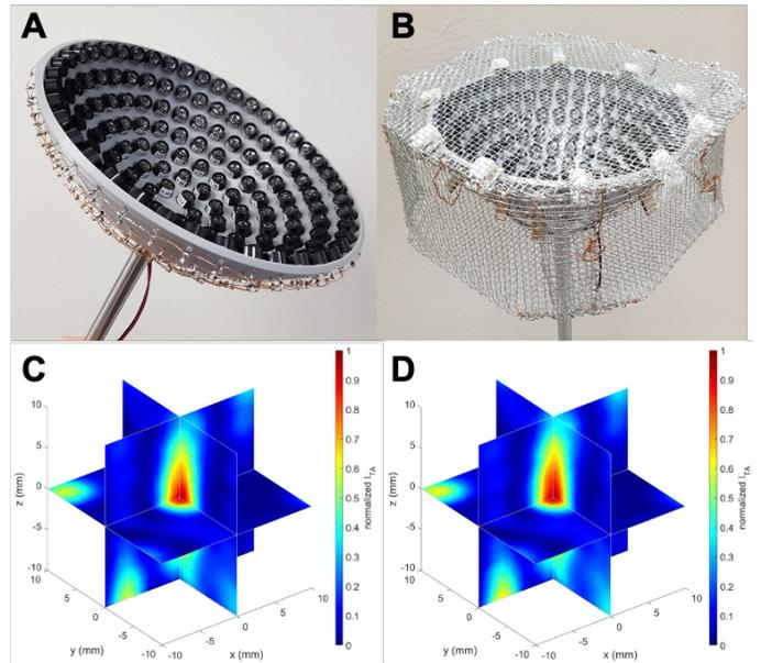
Fig. 1. Our ultrasonic haptic device. A dish-like array carries 168 elements shown in photographs without (A) and with (B) a Faraday cage. Respective graphs illustrate normalized sound intensity distributions in each case (C) and (D) underneath.
