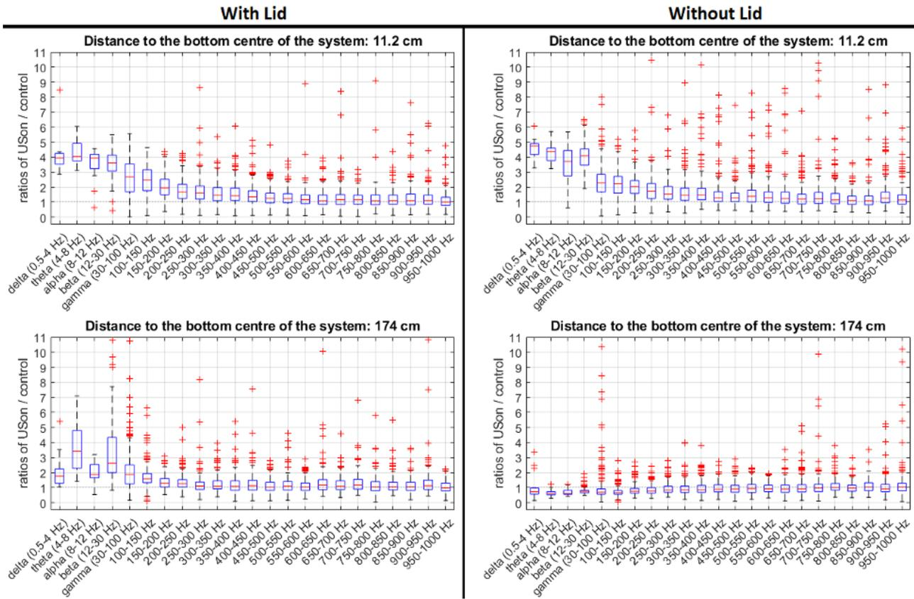
Fig. 3. Graphs of power spectral density ratios for magnetic field strength shown with the magnetometer placed above the system.
