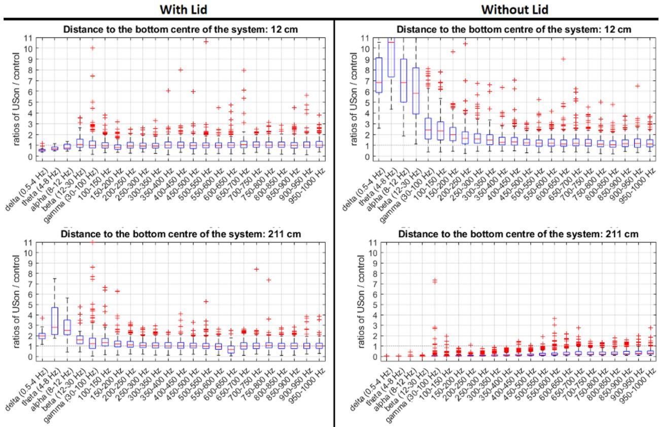
Fig. 2. Graphs of power spectral density ratios for magnetic field strength shown with the magnetometer placed to the side of the system.
