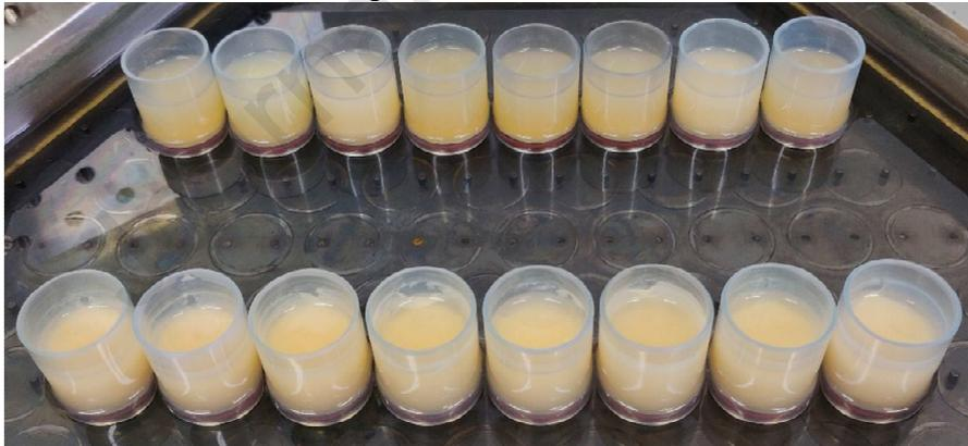
Fig. 3. Lubricant chambers in water bath of SuperCTPOD after 0.6 million cycles at 20 °C showing typical opaque appearance and yellow-brown color of used serum lubricant. Upper row ACS, lower row BCS.
