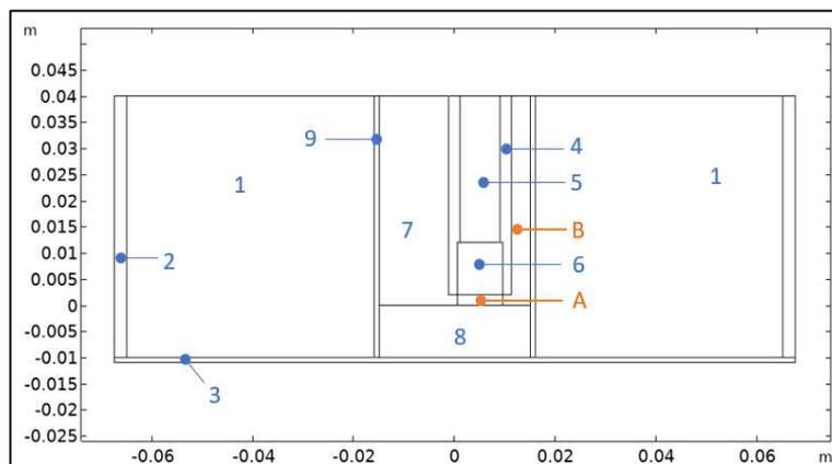
Fig. 1. Schematic of CTPOD thermal model. 1 Water bath, 2 Wall of water bath, 3 Base of water bath, 4 Polyacetal sleeve, 5 Pin guiding and loading shaft made from stainless steel, 6 Polyethylene pin, 7 Lubricant, 8 CoCr disk, 9 Stainless steel casing, A pin subsurface thermocouple, B lubricant thermocouple.
