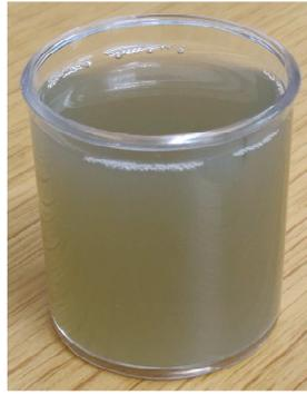
Fig. 6. Greenish color of used BCS lubricant of SuperCTPOD test at 37 °C.
