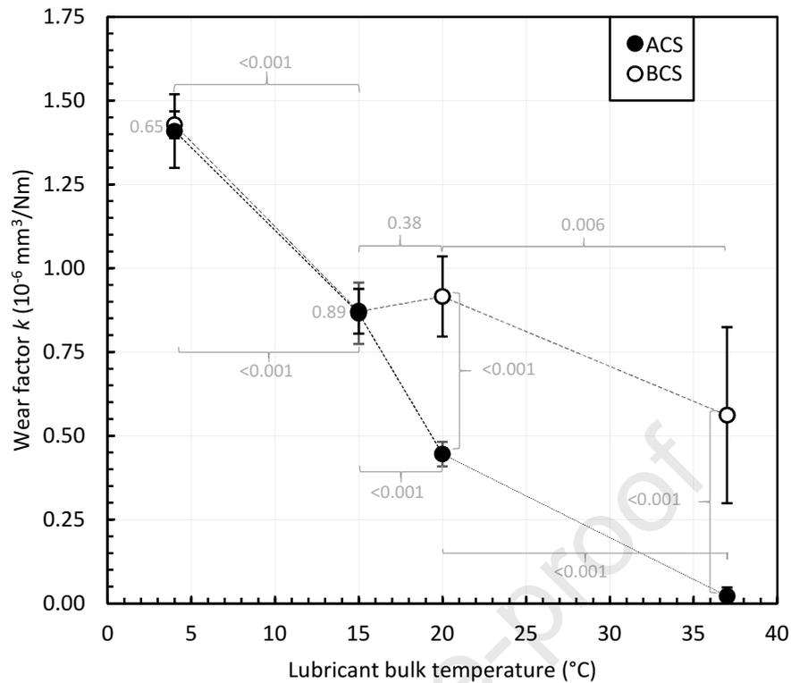
Fig. 2. Variation of VEXLPE wear factor (mean  $\pm$  SD) with lubricant bulk temperature in SuperCTPOD tests. Numbers indicate p-values of t-test between two test conditions.
