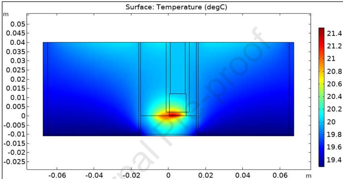
Fig. 8. Computed temperature distribution in 20 °C CTPOD test.
