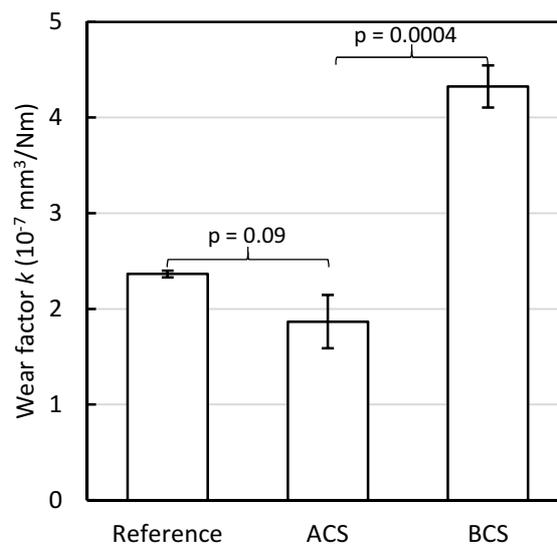
Fig. 9. Wear factors of VEXLPE liners (mean  $\pm$  SD) in HUT-4 hip simulator tests of  $3 \times 550\,000$  cycles duration. Reference is from [30], in which test duration was  $3 \times 320\,000$  cycles and lubricant was ACS. Lubricant bulk temperature was  $27\text{ }^{\circ}\text{C}$ .
