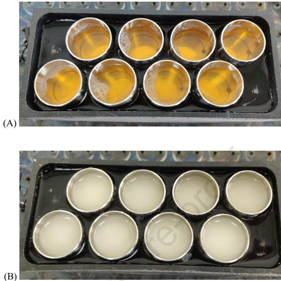
Fig. 4. Plastic ‘sub-bath’ of SuperCTPOD through which refrigerated water (inlet temperature 1 °C to 2 °C) was circulated in cold testing. Note thin stainless steel lubricant chambers for improved heat conductivity, as estimated friction power was 0.7 W per test station. Test disk formed bottom of chamber. (A) Before start ACS was transparent, (B) after 0.6 million cycles (1 week) at 2 °C to 4 °C, ACS had turned opaque and white.
