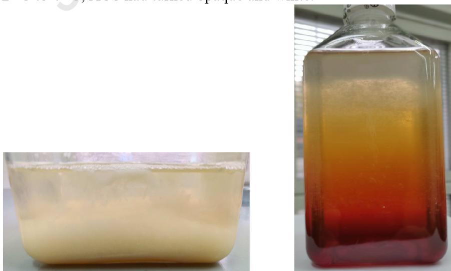
Fig. 5. Flocculation in used ACS lubricant of SuperCTPOD test at 4 °C (left), and for comparison, bottle of fresh, thawed, unshaken alpha calf serum (right).
