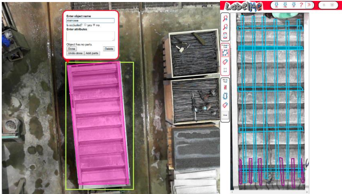
Figure 15. Manual labeling the data. The left image shows the way we labeled the staircase in the image. The right image shows the rebars labeling output.
