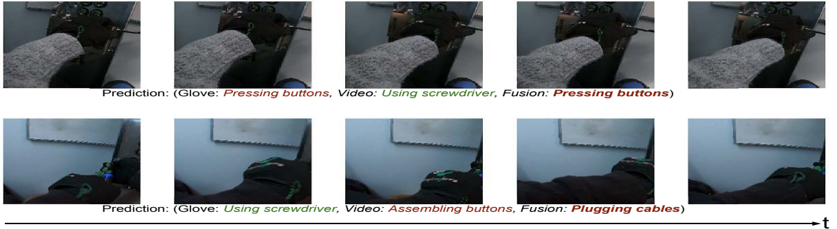
Figure 11: Failure examples of the fusion visualized for the Using screwdriver samples. (top row) The hand-screwdriver interaction is recognized by the video-based network, but the fusion model is persuaded by the glove recordings. (bottom row) Fusion model fails to use the hands dynamics.
