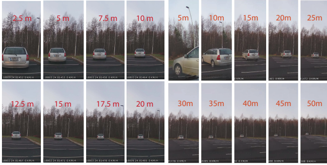
(a) Occupation of The Vehicle in Front in Photos Taken from Different Distances Away (b) Occupation of The Target of Interest in Photos Taken from Different Distances Away
