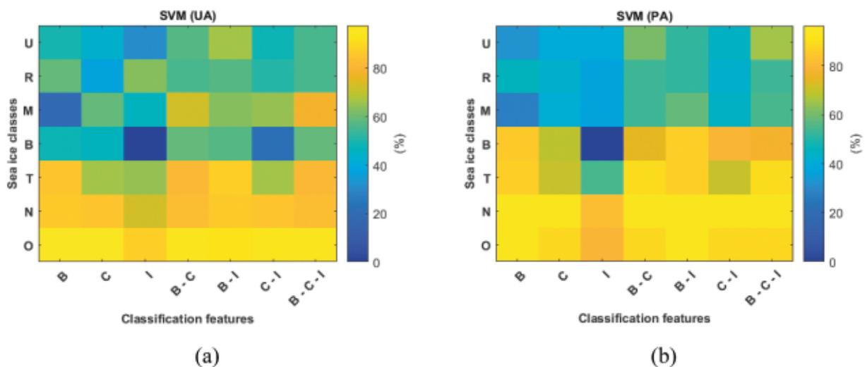
**Figure 9.** (a) UA and (b) PA in SVM classifier for water and sea ice classes (U = Undeformed ice, R = Ridged ice, M = Moderately deformed ice, B = Brash ice, T = Thick level ice, N = New ice, O = Open water), classification features (B = Backscatter-intensity, C = Coherence-magnitude, I = InSAR-phase).
