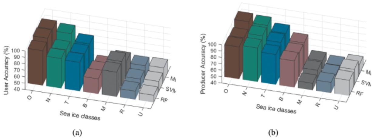
**Figure 5.** (a) User accuracy and (b) producer accuracy of RF, ML and SVM classified map based on backscatter-intensity & coherence-magnitude & InSAR-phase for water and sea ice classes (U = Undeformed ice, R = Ridged ice, M = Moderately deformed ice, B = Brash ice, T = Thick level ice, N = New ice, O = Open water).
