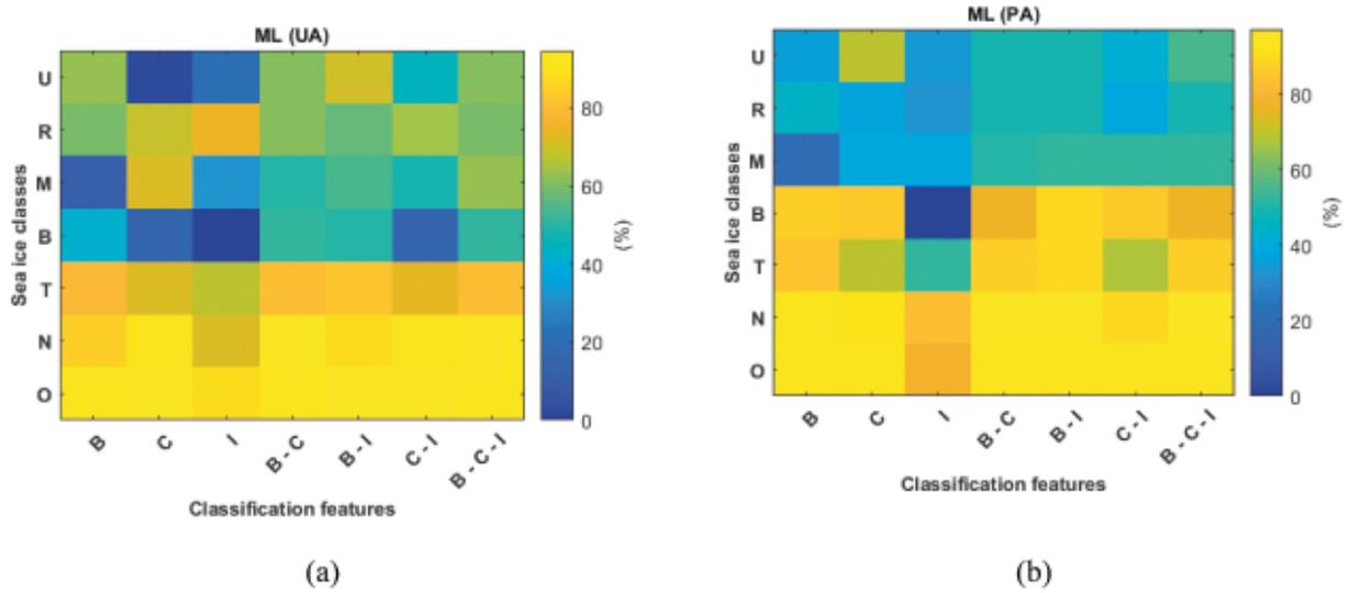
**Figure 8.** (a) UA and (b) PA in ML classifier for water and sea ice classes (U = Undeformed ice, R = Ridged ice, M = Moderately deformed ice, B = Brash ice, T = Thick level ice, N = New ice, O = Open water), classification features (B = Backscatter-intensity, C = Coherence-magnitude, I = InSAR-phase).
