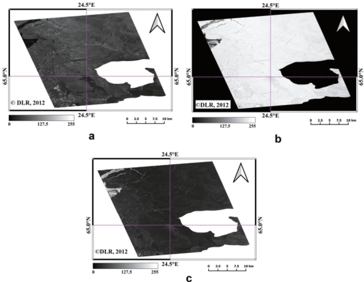
**Figure 2.** TanDEM-X image features: (a) backscatter intensity; (b) coherence-magnitude; (c) InSAR-phase. The image was acquired 30 March 2012. Land mask was applied. The features were linearly stretched to [0;255] dynamic range.
