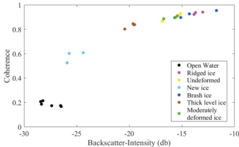
**Figure 10.** Coherence-magnitude and backscatter-intensity values of water and sea ice types for plots using pair HH-bistatic data for coherence-magnitude calculation and HH-bistatic data for backscatter-intensity calculations.
