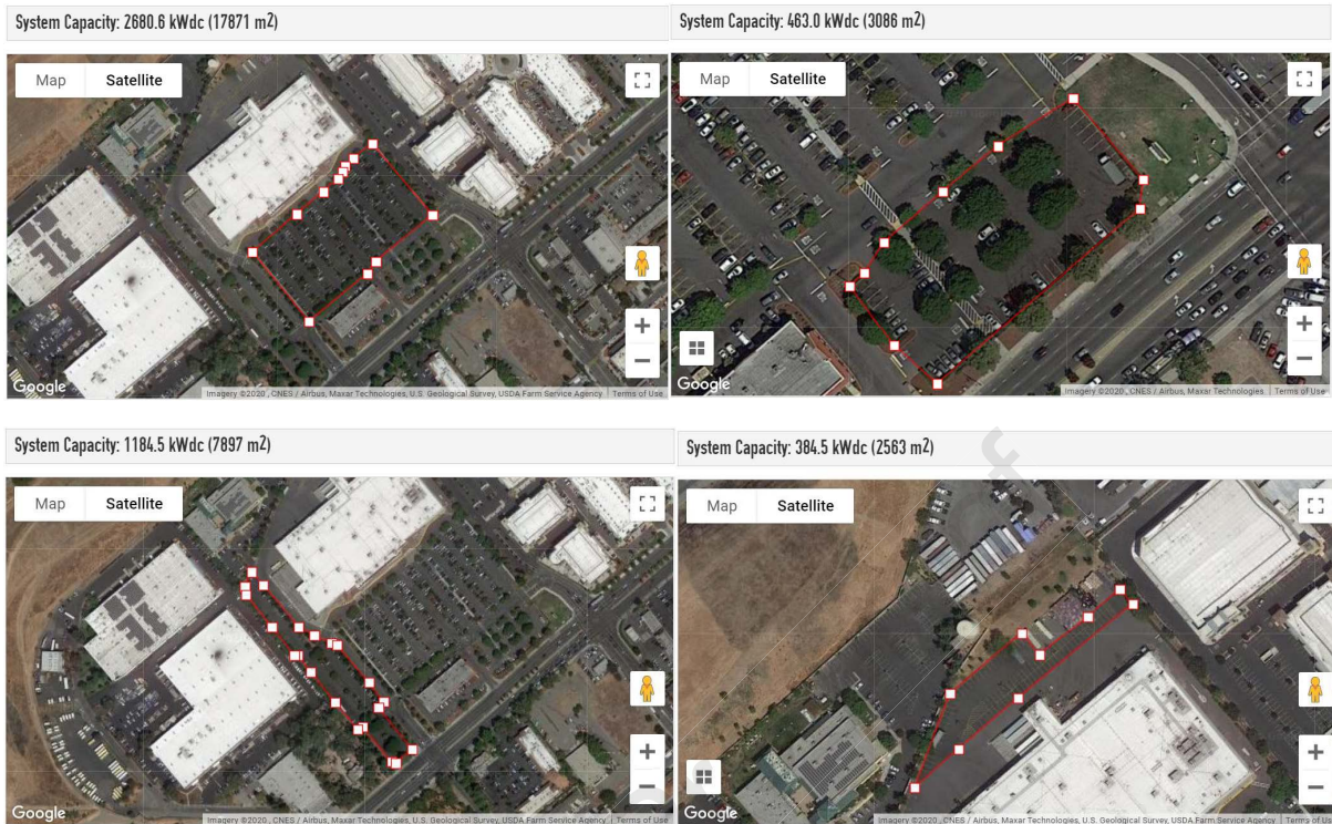
Figure 2. System capacity for Walmart 1, Walmart Supercenter, 31,417 m 2 total area, 4,712.6 kW dc potential PV.
