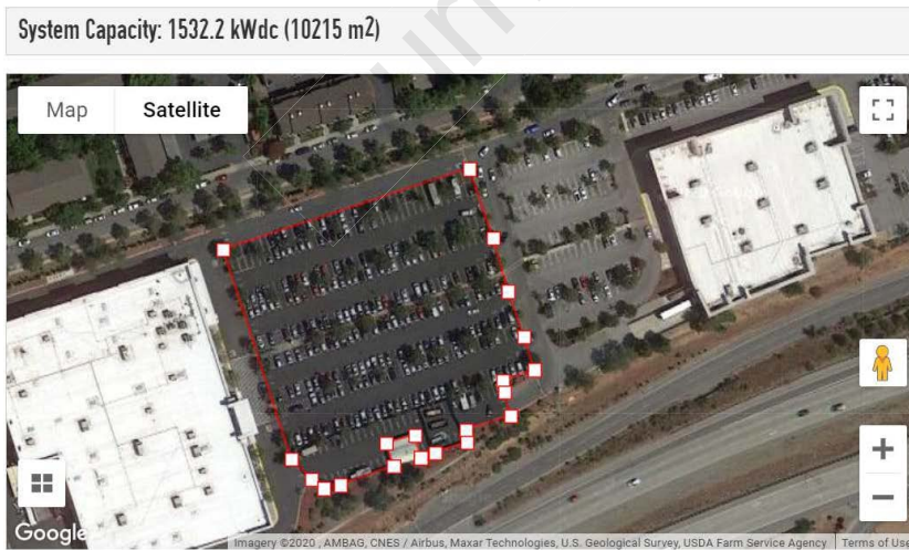
Figure 3. System capacity for Walmart 2 – Walmart Supercenter, 10,215 m 2 total area and 1,532.3 kW dc potential PV.
