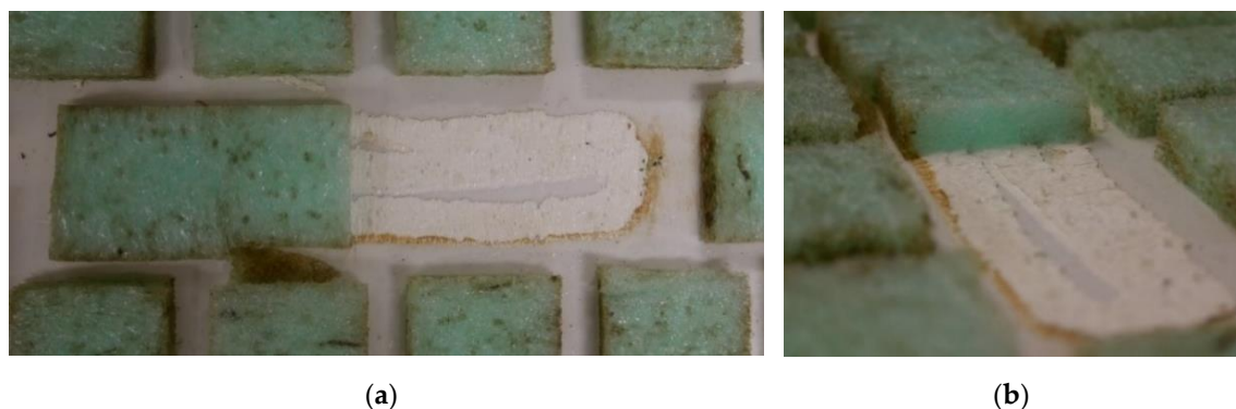
Figure 1. Cutaway view showing adhesive underneath foam attached to a Si-based flexible photovoltaic (PV) module: (a) top view and (b) orthogonal view.
