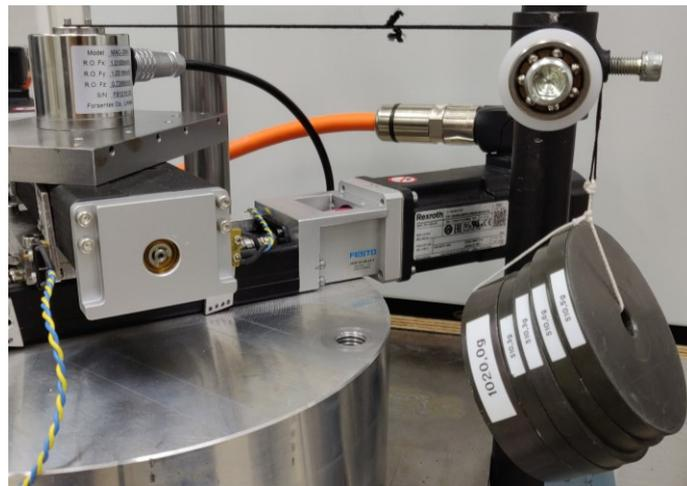
Figure 1(e). Checking version 2 calibration in  $x$  direction with 30 N load.
