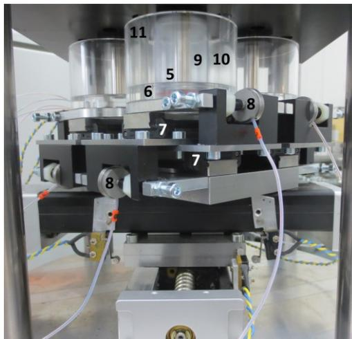
Figure 1(b). Friction measurement assembly, 5 pin, 6 disk, 7 linear bearing, 8 button load cell, 9 lubricant chamber, 10 water bath, 11 hose for circulating cooling/heating water.
