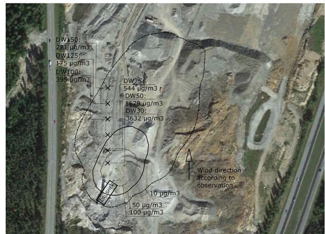
**Fig. 5** Modelled concentration contours of the model C5 and the measured  $\text{PM}_{10}$  concentrations near two stages crushing. X is the measurement location in the downwind (DW) direction. Aerial photograph: Google Earth Pro
