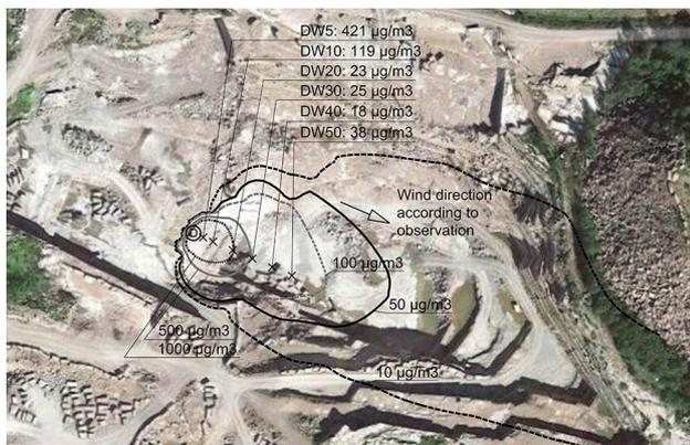
**Fig. 4** Modelled concentration contours of the model D2 and the measured  $\text{PM}_{10}$  concentrations near the drilling. (D) denotes the drill. X is the measurement location in the downwind (DW) direction. Aerial photograph: Google Earth Pro
