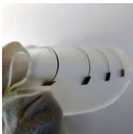
Fig. 4. Flexible thiol-ene electrodes. Thiol-ene (thickness 0.5 mm) is bent over a radius of 2 mm resulting in negligible change in resistances of the electrodes.
