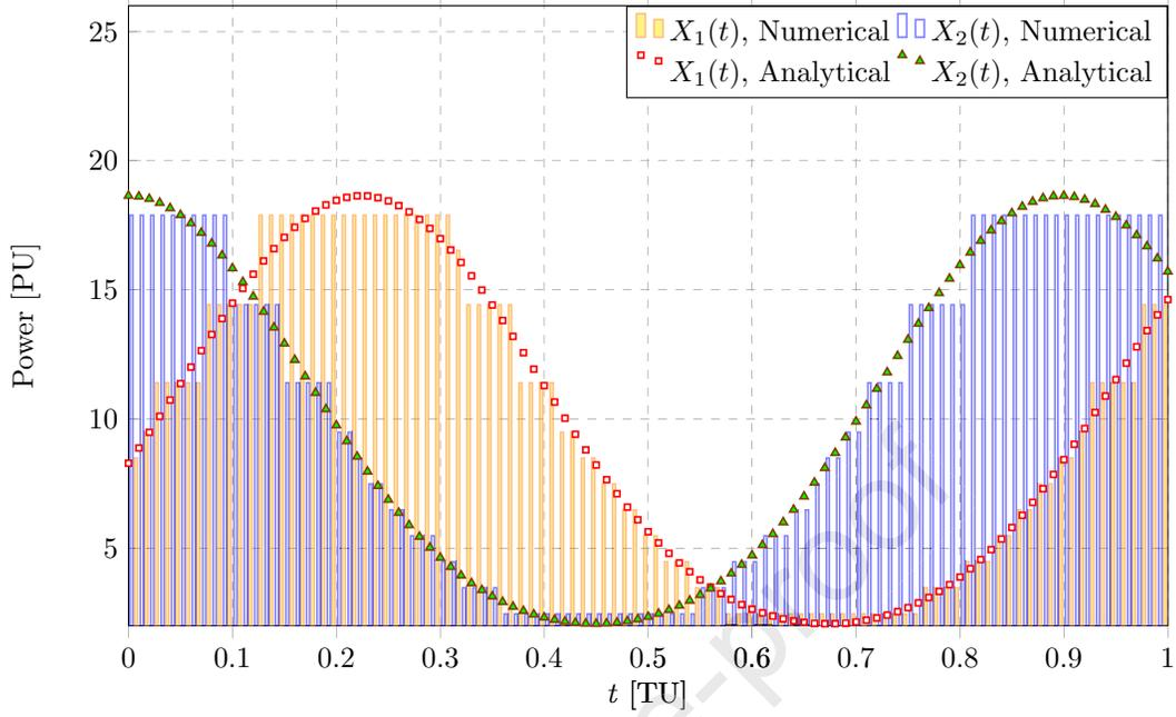
Figure 11: Discharging schedules obtained numerically and analytically with  $E_0 = 20[\text{EU}]$ . Mismatch depends on discretization step size  $\Delta t$  and number of linear segments  $Q$ , used to approximate Eq. (3). In this scenario  $\Delta t = 0.01$  and  $Q = 21$ .
