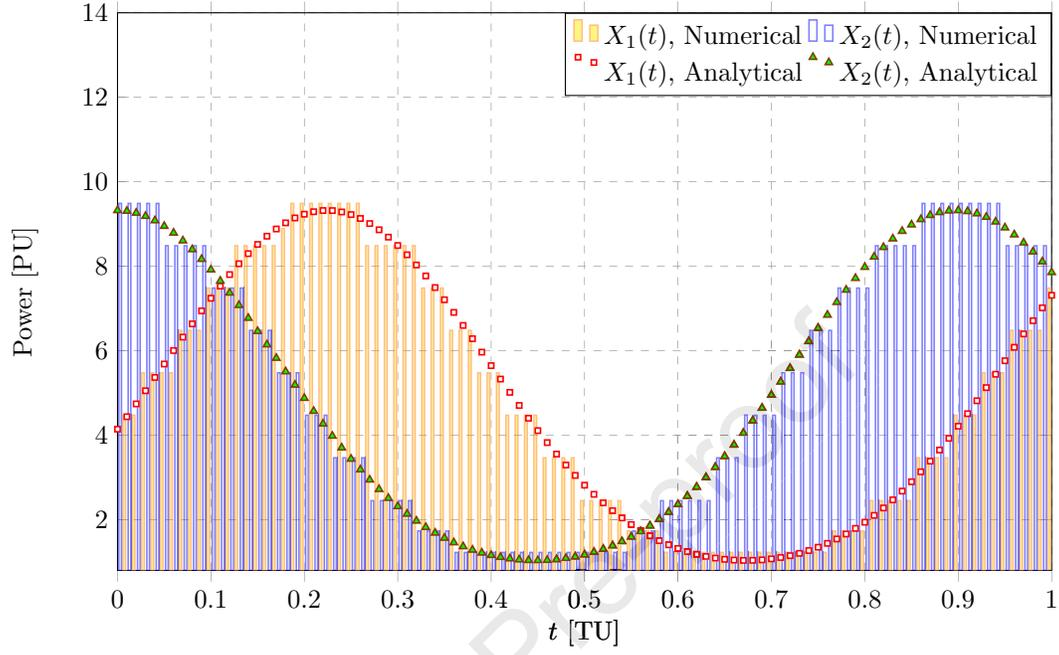
Figure 10: Discharging schedules obtained numerically and analytically with  $E_0 = 10[\text{EU}]$ . Mismatch depends on discretization step size  $\Delta t$  and number of linear segments  $Q$ , used to approximate Eq. (3). In this scenario  $\Delta t = 0.01$  and  $Q = 21$ .
