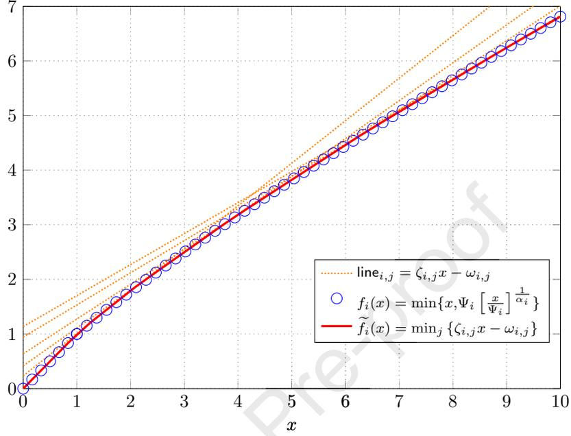
Figure 2: Piece-wise linear approximation of Eq. (3), with  $\Psi_i = 1$ ,  $\alpha_i = 1.2$ ,  $\forall i$ ,  $Q = 6$ . The dotted lines represent tangents to function  $f_i(x)$ , the solid line is the point-wise minimum across  $Q = 6$  lines. The original model is plotted with circular marks.
