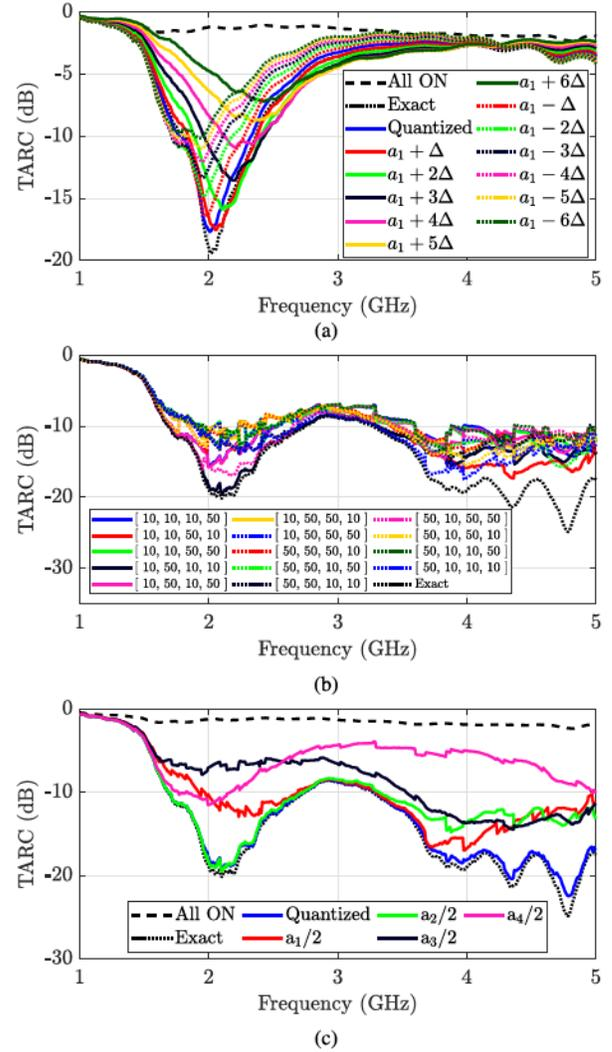
Fig. 4. (a) Effect of amplitude variations for 2-GHz case: Feed 1 amplitude  $a_1$  is analyzed for various error steps where  $\Delta = \pm 0.1$  V. (b) Effect of simultaneous error in all amplitudes  $a_1$ – $a_4$  with two different error sizes: 10% and 50%. (c) Effect of amplitude variations on antenna TARC profile for  $a_i/2$  such that  $a_{i \neq j}$  and  $\varphi_i$  are intact, where  $i, j = 1, \dots, 4$ .
