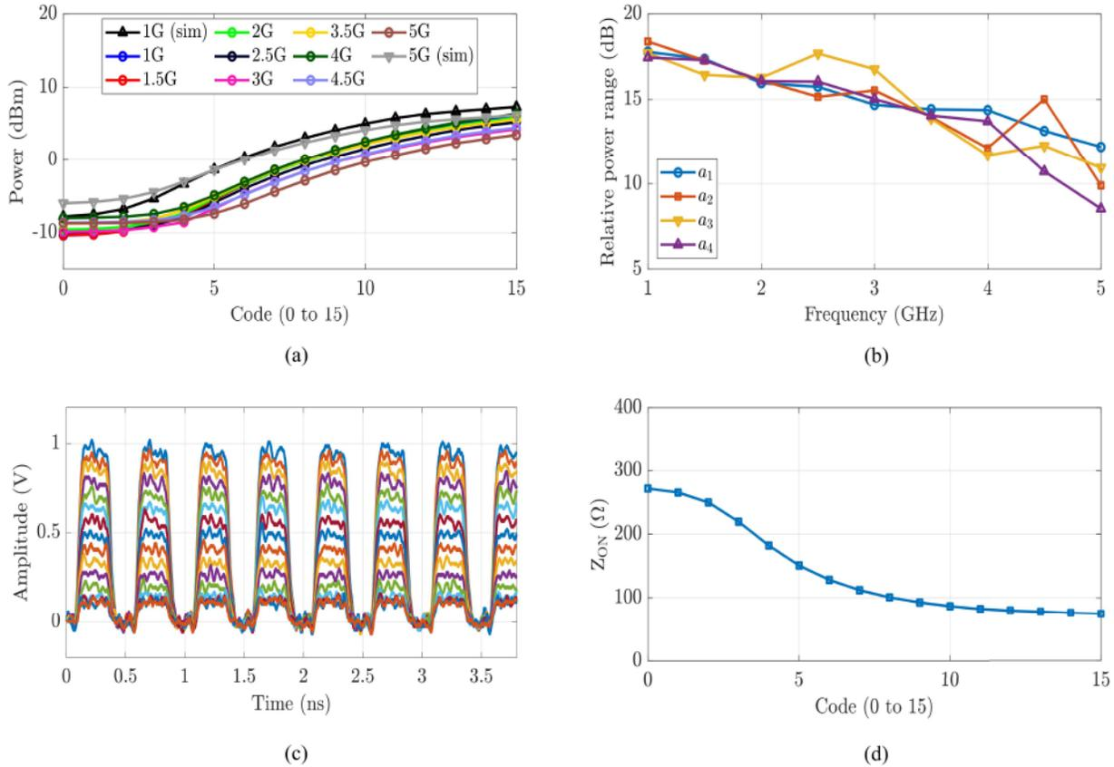
Fig. 8. (a) Measured power scaling of a single transmitter output from 1.5 to 5 GHz. (b) Measured output power ranges of all four IC outputs  $O_1$ – $O_4$ . (c) Measured amplitude scaling performance at 2 GHz for one single amplitude tuning block. (d) Simulated turn-on resistance of class-d device for scaling of  $V_{LDO}$ .
