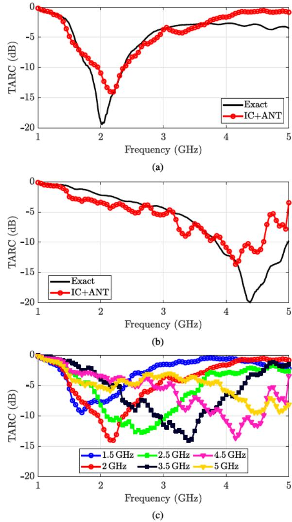
Fig. 11. Measured tuning performance of antenna cluster at (a) 2 and (b) 4.5 GHz. (c) Measured wideband antenna tuning performance across the spectrum.
