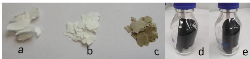
Figure 5. Cellulosic samples before and after degradation with gaseous HCl. a) Untreated Whatman 1 paper, b) Whatman 1 paper after 1.5 h treatment time with 100 kPa HCl pressure, c) Whatman 1 paper after 68 h treatment time with 100 kPa HCl pressure, d) Whatman 1 with 10 w-% water content after 72 h treatment, e) Whatman 1 with 20 w-% water content after 72 h treatment.
