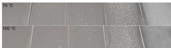
**Fig. 5** EHEC–MFC films dried on a glass plate at 70 °C and 100 °C. From the left: pure EHEC, EHEC:MFC with ratios of 25:75, 50:50 and 25:75, and pure MFC
