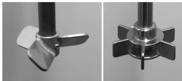
**Fig. 2.** Impellers used in the test work. A pitched blade turbine, diameter 50 mm (left). A radial flow turbine, diameter 45 mm (right).
